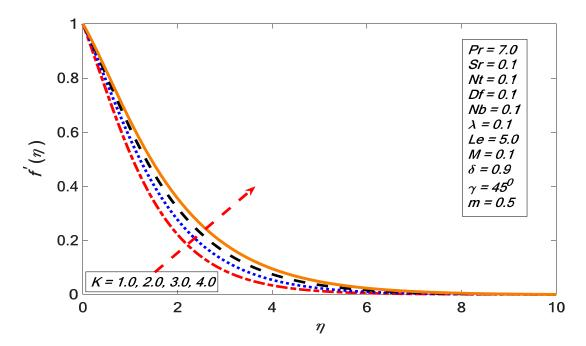
Figure 6. Variations in the velocity profile for several values of *K*.
