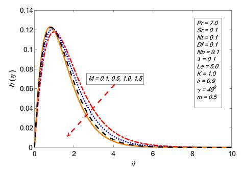
Figure 3. Variations in the angular velocity for several values of *M*.
