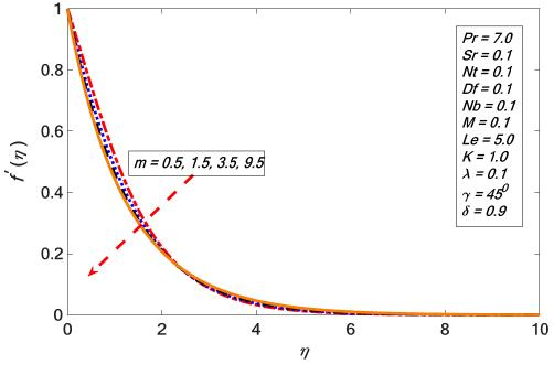
Figure 17. Variations in the velocity profile for several values of *m*.
