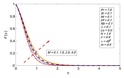
Figure 4. Variation in the temperature profile for several values of *M*.
