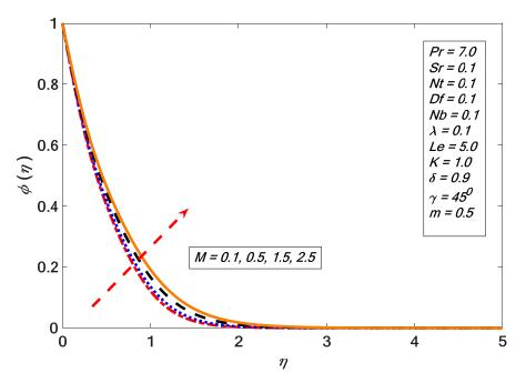
Figure 5. Variations in the concentration profile for several values of *M*.
