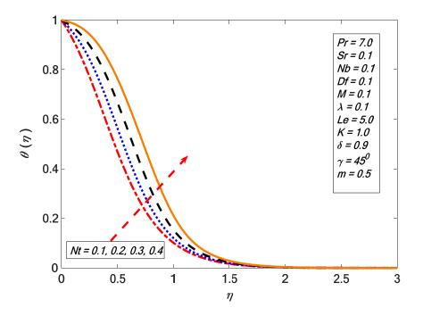
Figure 22. Variations in the temperature profile for several values of *Nt*.
