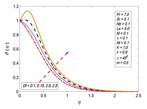
Figure 26. Variations in the temperature profile for several values of *Df*.
