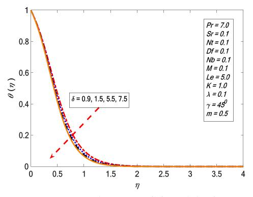
**Figure 15.** Variations in the temperature profile for several values of  $\delta$ .
