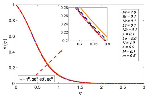
**Figure 9.** Variations in the temperature profile for several values of  $\gamma$ .
