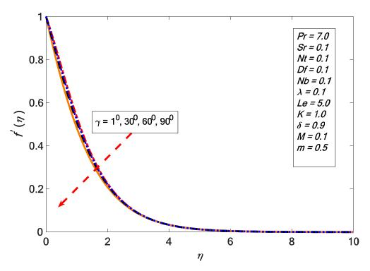
**Figure 8.** Variations in the velocity profile for several values of  $\gamma$ .
