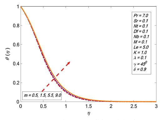
**Figure 18.** Variations in the temperature profile for several values of *m*.
