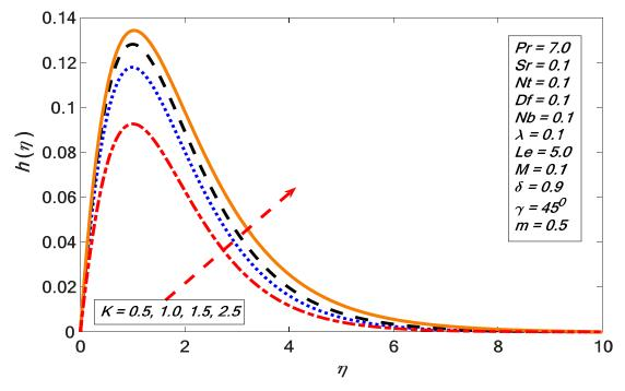
Figure 7. Variations in the angular velocity profile for several values of *K*.
