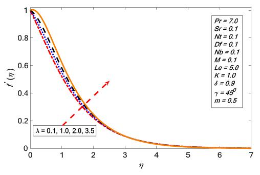
**Figure 11.** Variations in the velocity profile for several values of  $\lambda$ .
