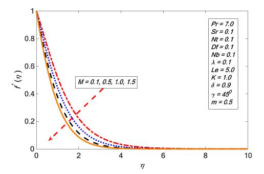
Figure 2. Variations in the velocity profile for several values of *M*.
