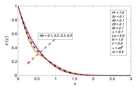
Figure 21. Variations in the concentration profile for several values of *Nb*.
