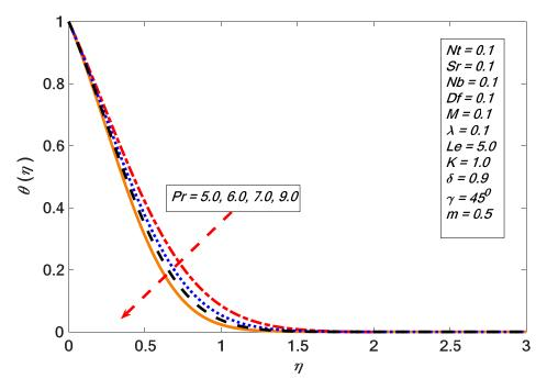
Figure 24. Variations in the temperature profile for several values of Pr.
