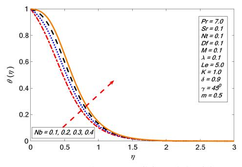
Figure 20. Variations in the temperature profile for several values of *Nb*.
