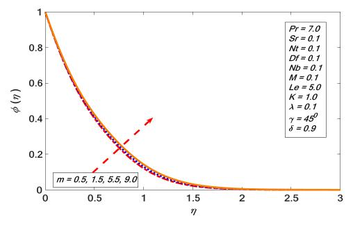
Figure 19. Variations in the concentration profile for several values of *m*.
