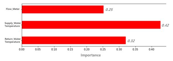
Figure 7. Gini importance of heating supply data.
