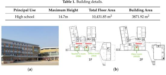
**Figure 1.** High school building used for this study: (**a**) View of High school; (**b**) Floor plan and sensor locations. (Name of the data points: Office room is HS3; Teacher's room is HS8; Classroom HS10.)
