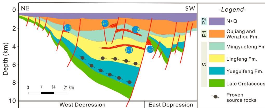
**Figure 12.** Schematic geological cross-section of the Lishui Sub-basin, and its proven and speculative plays. Note that all belong to the Yueguifeng–Lingfeng Petroleum System (!). Line location is indicated in Figure 11. All the red lines are normal faults; S = syn-rift; P1 = early post-rift; P2 = late post-rift; i-1 = Lingfeng structural (proven); i-2 = Mingyuefeng structural (proven); i-3 = Basement structural–stratigraphic (proven); ii-1 = Oujiang structural (speculative).
