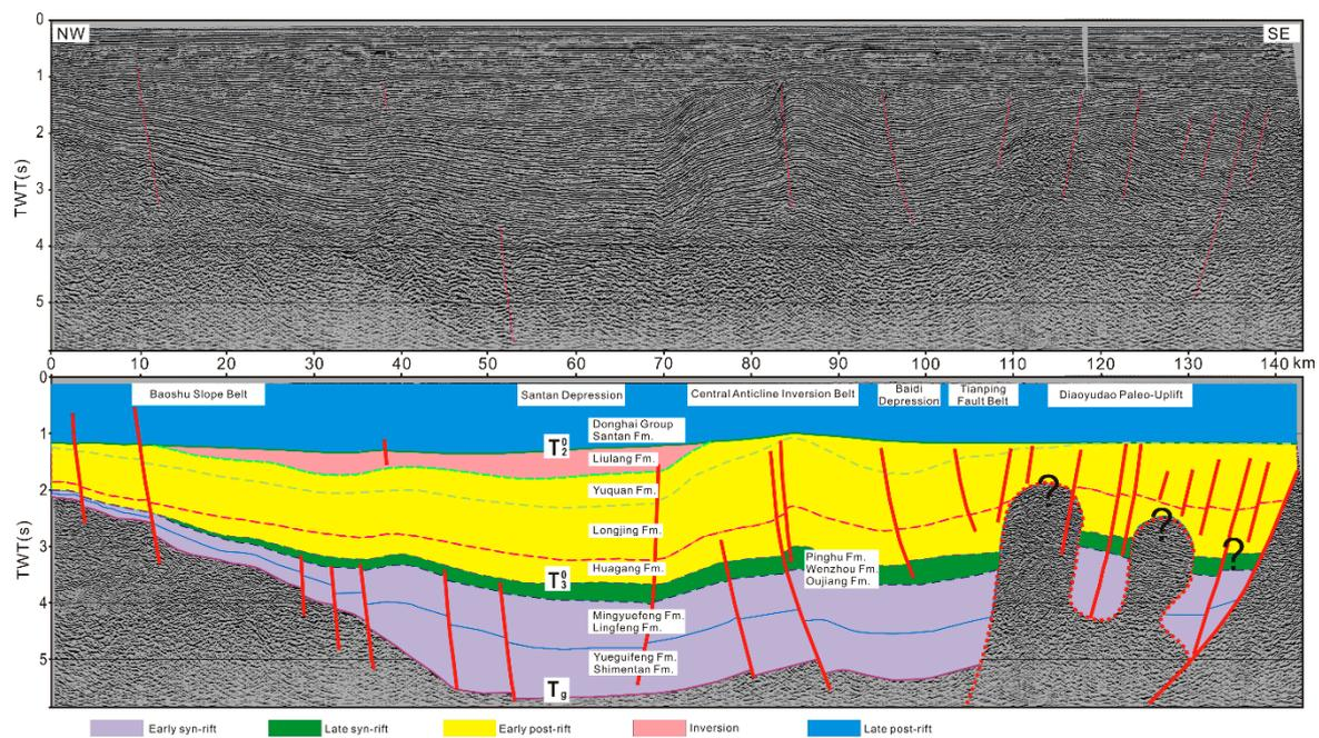
**Figure 7.** Xihu Sub-basin tectonic cross-section (seismic line location is indicated in Figure 6). The seismic horizons can be referred to Figure 3. Question marks indicate uncertainties in the interpretation.
