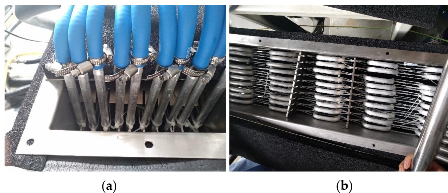
Figure 2. Photographs of the ice storage container (a) and coil-plate heat exchanger (b).
