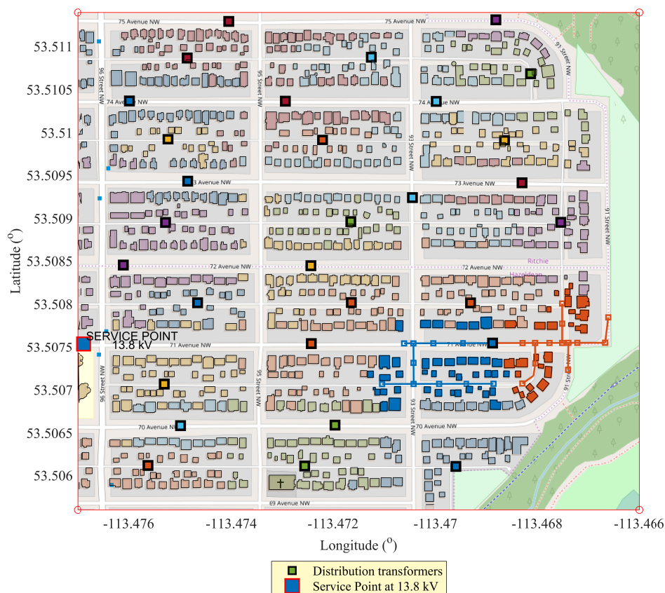
Figure 3. Case study 1: Low voltage distribution network, where distribution transformers and end users are represented with different colors depending on the cluster.
