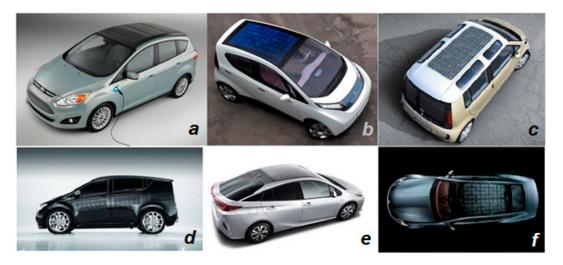
**Figure 1.** Vehicles with photovoltaic (PHV) battery: (a) Ford C-MAX Solar Energy concept; (b) Pininfarina B Zero; (c) Volkswagen Space Up Blue (hydrogen-powered); (d) Sono Sion electric vehicle; (e) Solar Roof as an option that Toyota offers to Prius and Auris hybrids; (f) Fisker Karma hybrid vehicle.
