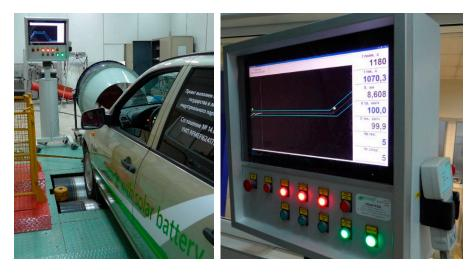
**Figure 10.** Laboratory tests of the developed electric vehicle (on the left: test at the bench with running drums in the driving cycle mode; on the right: speed monitor).
