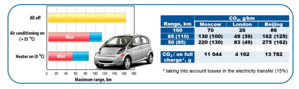
Figure 3. Recalculation of electricity consumption by an electric vehicle to the CO<sub>2</sub> emissions.
