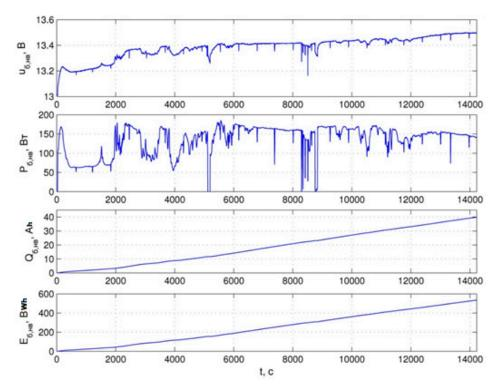
**Figure 11.** Readings of operation of the PHV system in the process of charging the buffer storage with solar energy.
