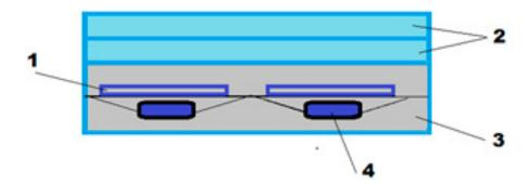
**Figure 8.** Photovoltaic converters system diagram (section): 1—PHV; 2—protective glazing; 3—filler compound; 4—bypass diode.
