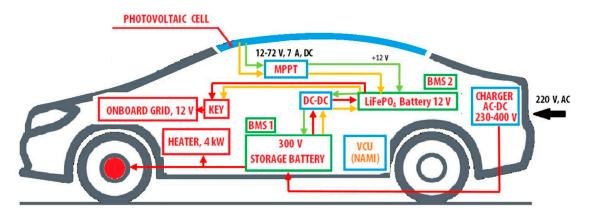
Figure 5. Scheme of the dual-circuit system of photovoltaic converters.
