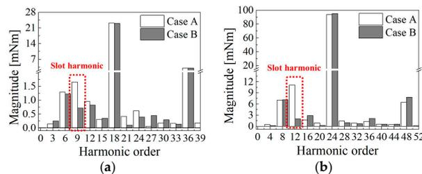
Figure 15. Cogging torque measurement of each motor for (a) 6p/9s IPM and (b) 8p/12s IPM.
