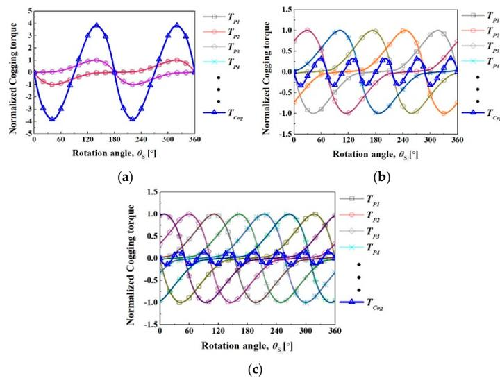
**Figure 3.** Cogging torque caused by multi poles rotation based on  $\theta_s$ : (a) cogging torque of 8p/12s, (b) cogging torque of 10p/12s, and (c) cogging torque of 14p/12s.
