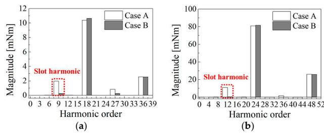
**Figure 8.** FEA results of cogging torque harmonic component according to each case: (a) 6p/9s IPM and (b) 8p/12s IPM.
