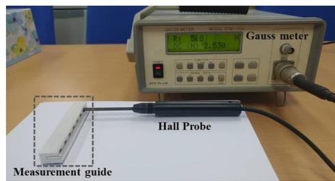
Figure 11. Gauss measurement of the magnet surface.
