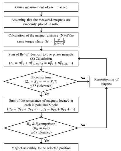
**Figure 5.** The workflow diagram of a method for mitigating slot harmonic cogging torque before rotor assembly.
