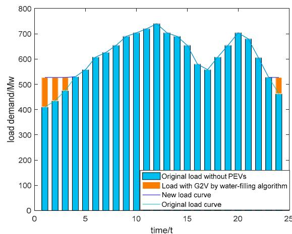
**Figure 8.** New 24-h load curve after valley filling.
