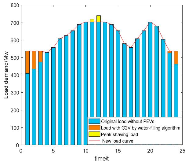
**Figure 10.** New 24-h load curve after valley filling and peak shaving.
