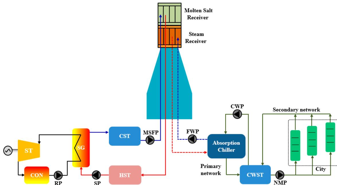
**Figure 5.** Solar power tower and DC system proposed by Marugán-Cruz et al., adapted from [30]. Note: CON—condenser; CST—cold storage tank; CWP—chilled water pump; CWST—chilled water storage tank; FWP—feed water pump; HST—hot storage tank; MSFP—molten salt feed pump; NMP—network main pump; RP—Rankine pump; SG—steam generator; SP—storage pump; ST—steam turbine.
