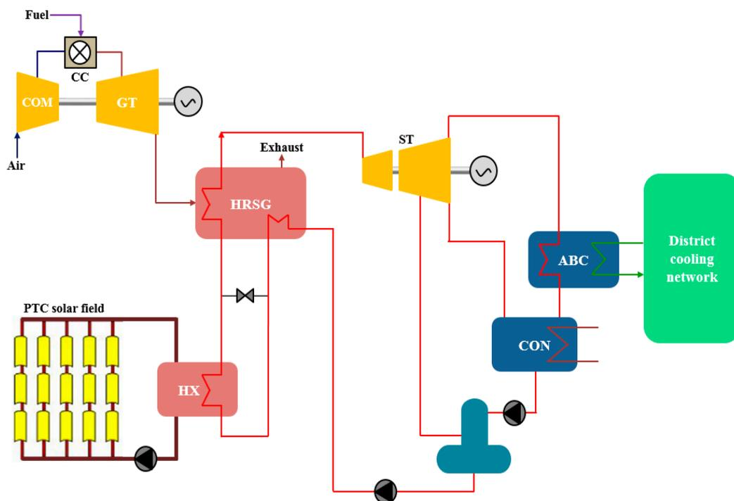
**Figure 6.** Solar combined cooling and power (SCCP) plant proposed by Perdichizzi et al., adapted from [31]. Note: ABC—absorption chiller; CC—combustion chamber; COM—compressor; CON—condenser; GT—gas turbine; HRSG—heat recovery steam generator; HX—heat exchanger, PTC—parabolic trough solar collector; ST—steam turbine.
