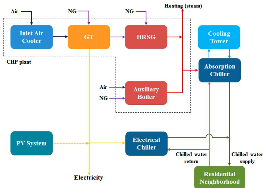
**Figure 3.** NG- and solar PV-powered tri-generation system proposed by Ondeck et al. for future residential neighborhoods in hot-climate regions, adapted from [28]. Note: CHP—combined heat and power; GT—gas turbine; HRSG—heat recovery steam generator; NG—natural gas; PV—photovoltaic.
