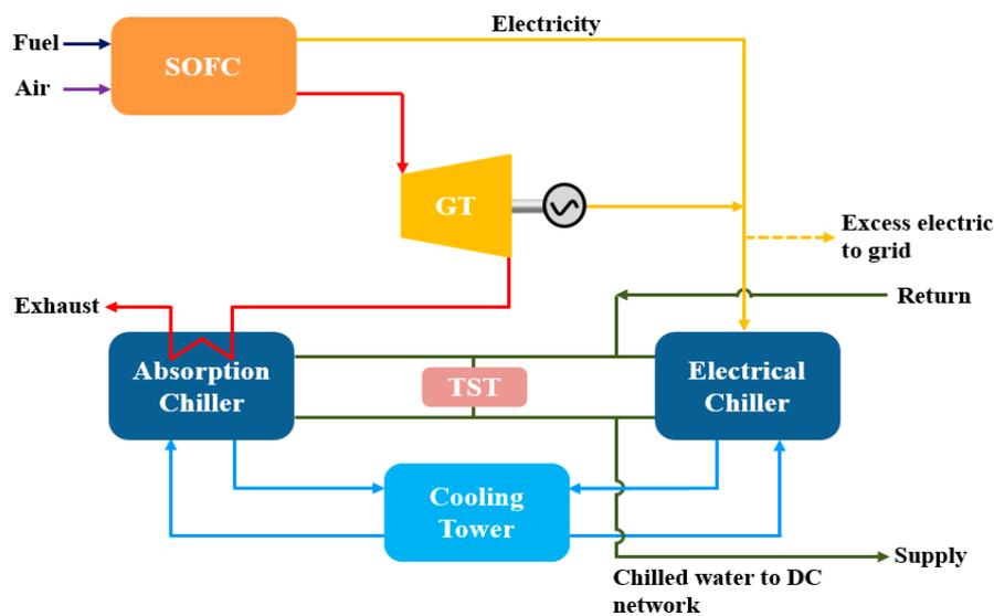
**Figure 4.** Integrated SOFC-GT and DC system proposed by Al-Qattan et al. for a new city in Kuwait, adapted from [6]. Note: GT—gas turbine; SOFC—solid oxide fuel cell; TST—thermal storage tank.
