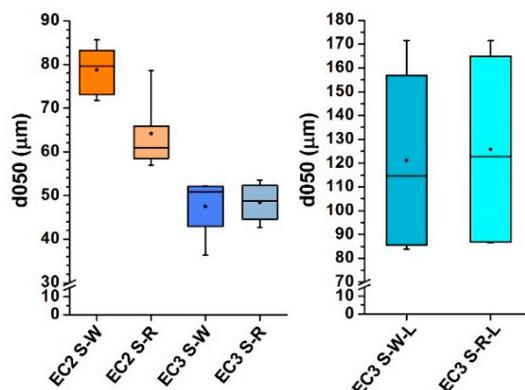
**Figure 12.** Mean value of particle size of soot (d050) for boilers of EC2 and EC3 for interval 8–11 h and 22 h. S-W: soot-walls; S-R: soot-ribs; L: long-lasting burning.
