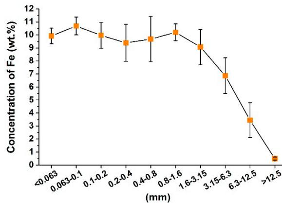
Figure 9. Dependence of concentration of Fe on particle size in ash.
