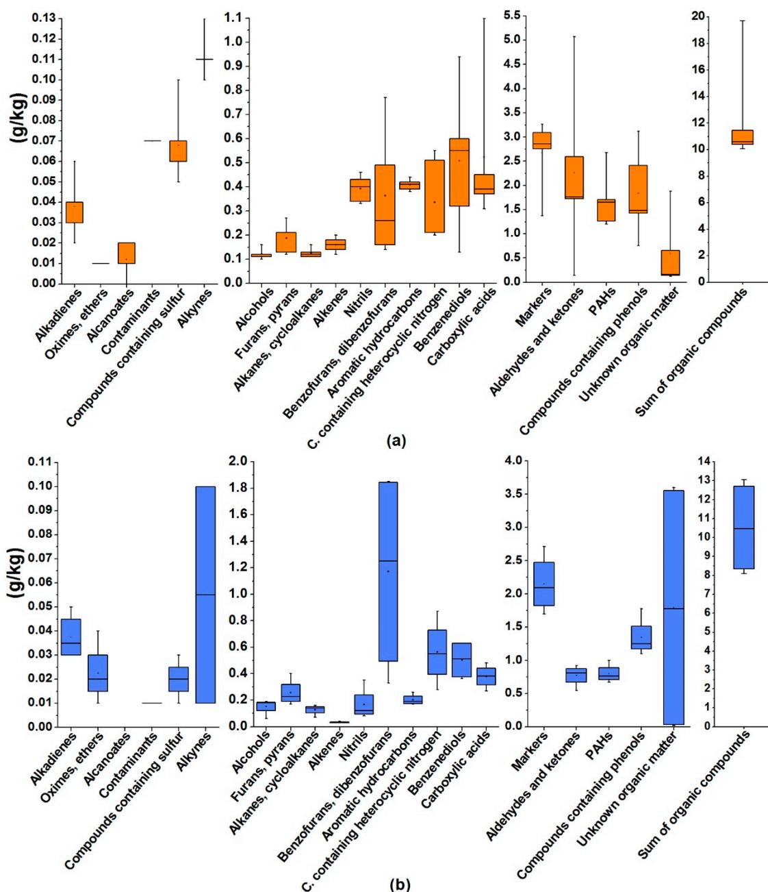
Figure 15. Organic compounds in pyrolysates: (a) boiler EC2; (b) boiler EC3.
