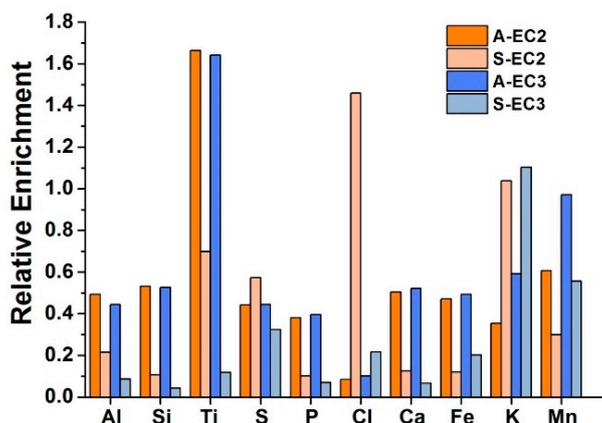
**Figure 5.** Relative enrichment for major elements in soot (S) and ash (A) from the combustion of peat briquettes in boilers EC2 and EC3.
