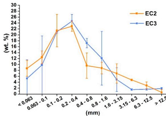
Figure 11. Comparison of the particle size distribution for ash particles from boilers of EC2 and EC3.
