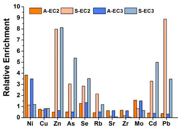
**Figure 6.** Relative enrichment for trace elements in soot (S) and ash (A) from the combustion of peat briquettes in boilers EC2 and EC3.
