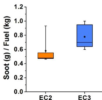
**Figure 1.** Boxplot-production of soot during peat briquettes combustion in boilers of emission class 2 and 3 (EC2 and EC3).
