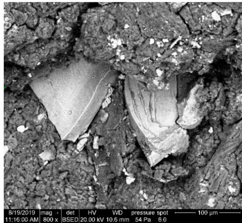
Figure 3. Quartz particles in peat briquettes.
