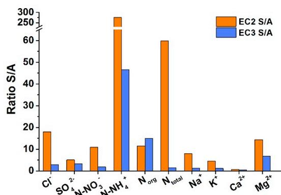
**Figure 14.** The proportion of leached ions from soot (S) and fly ash (A) for boilers of emission classes EC2 and EC3.
