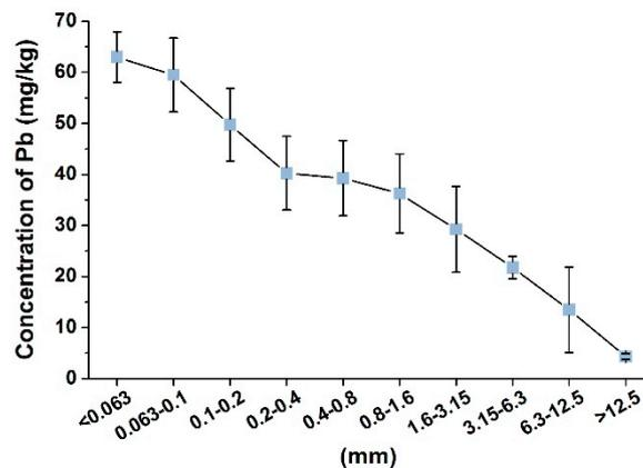
Figure 10. Dependence of concentration of Pb on particle size in ash.
