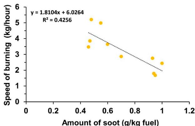
**Figure 2.** Relationship between amounts of produced soot from 1 kg of peat briquettes and speed of burning.
