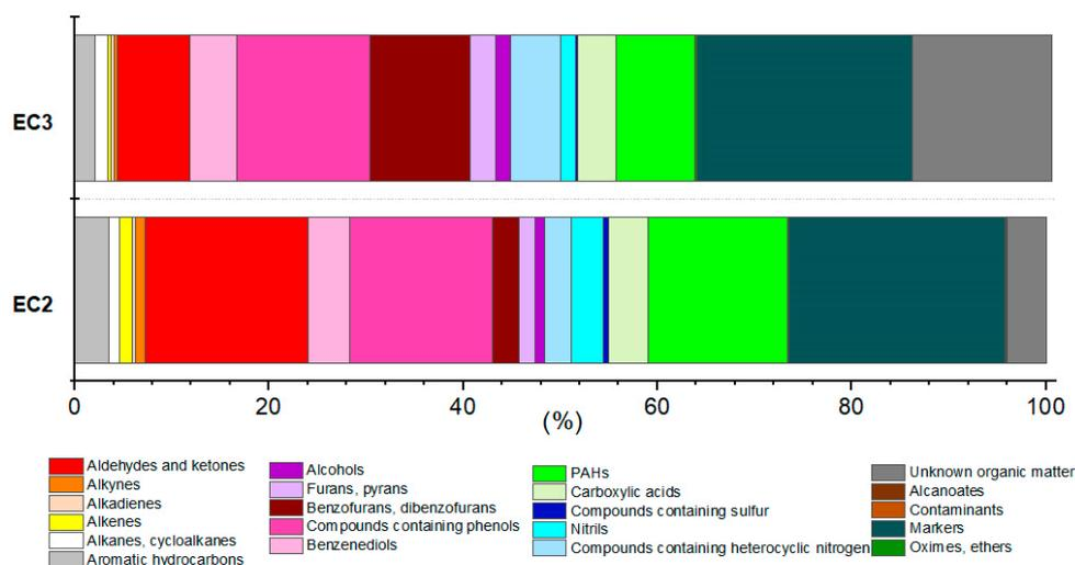
**Figure 16.** Percentages of groups of organic compounds in soot from boilers of emission class 2 and 3 (EC2 and EC3).
