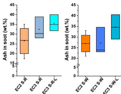
**Figure 13.** Content of ash in soot from the combustion of peat briquettes. S-W: soot-walls, S-R: soot-ribs, L: long-lasting burning.
