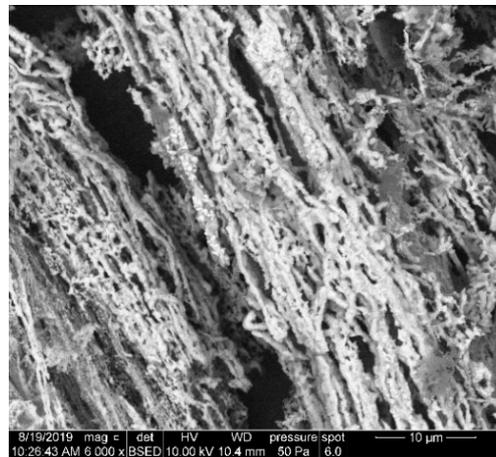
Figure 4. The character of char (calcified fibre) from the combustion of peat briquettes.
