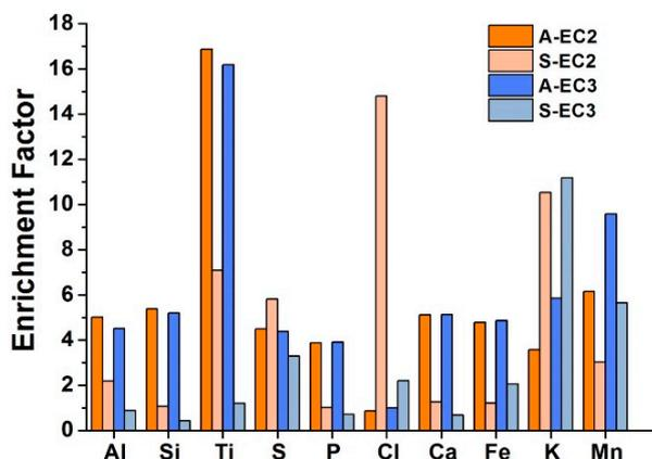
**Figure 7.** Enrichment factor (EF) for major elements in soot (S) and ash (A) from the combustion of peat briquettes in boilers EC2 and EC3.
