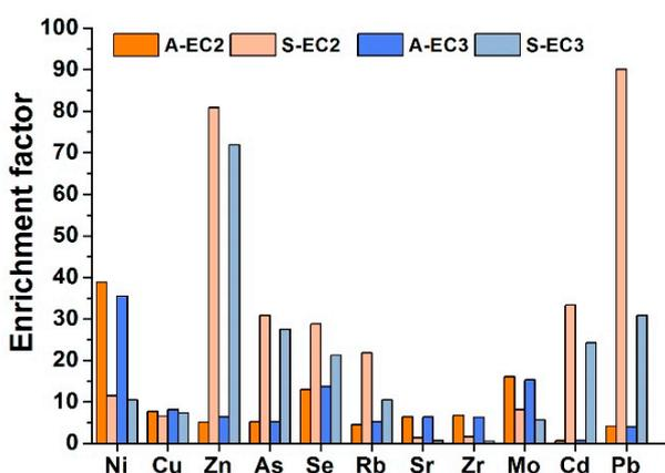
**Figure 8.** Enrichment factor for trace elements in soot (S) and ash (A) from the combustion of peat briquettes in boilers EC2 and EC3.
