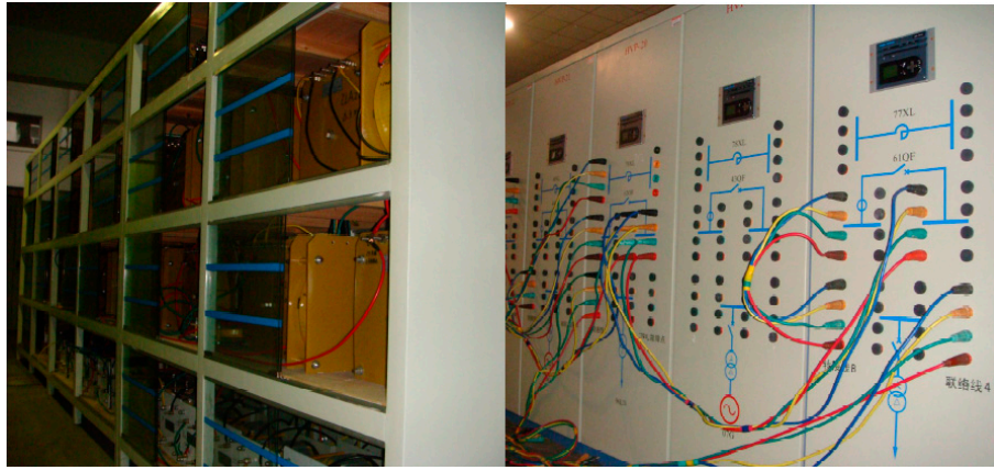
Figure 3. Traditional \pi -shape physical model of the three-phase transmission line.
