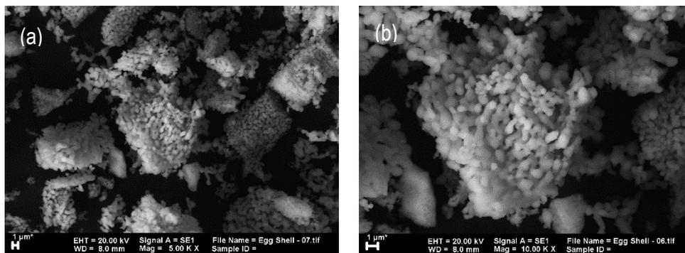
**Figure 4.** The SEM morphology of eggshell catalysts powder with magnification of (a) 5000× (b) 10,000×.
