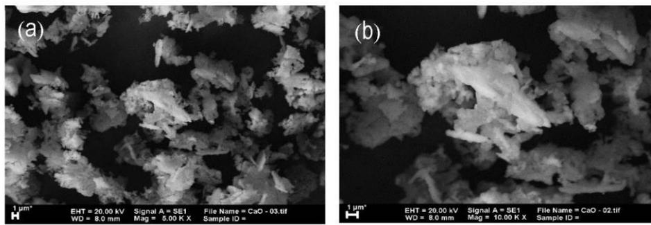
**Figure 3.** The SEM morphology of CaO-KOH catalysts powder with magnification of (a) 5000× (b) 10,000×.
