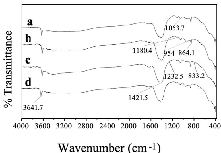
**Figure 1.** Fourier-transform infrared spectrometry (FT-IR) spectra of Potassium Hydroxide (KOH)-impregnated eggshell samples at various KOH concentrations (wt%): (a) 10%, (b) 15%, (c) 20%, and (d) 25% at 800 °C for 5 h.
