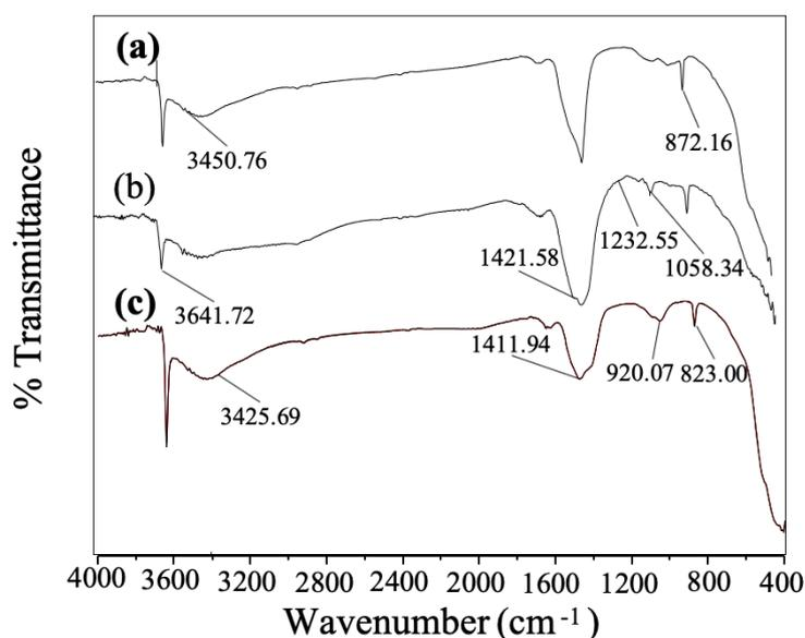
**Figure 2.** FT-IR spectra of (a) KOH-CaO, (b) KOH-impregnated eggshell, and (c) eggshell calcined at 800 °C for 5 h.
