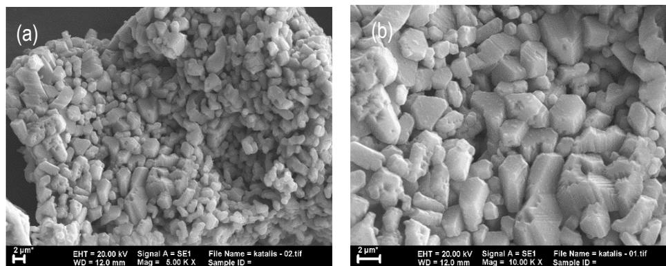
**Figure 5.** The SEM morphology of KOH-impregnated eggshell catalysts powder with magnification of (a) 5000× (b) 10,000×.
