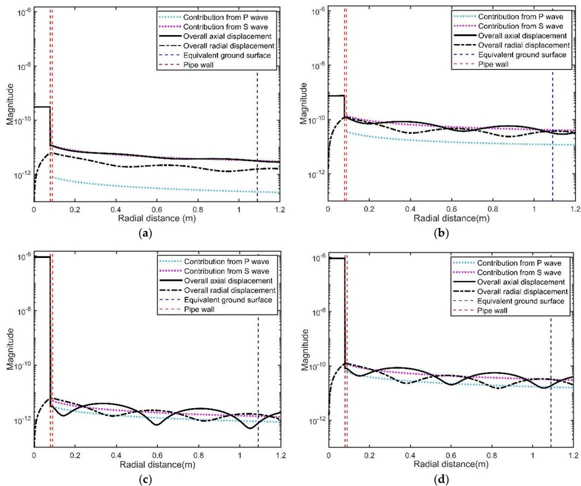
**Figure 5.** Displacement profiles in radial direction resulting from  $s = 1$  waves, for the pipes buried in soil A: (a) cast iron water pipe; (b) PVC water pipe; (c) cast iron gas pipe; and (d) PVC gas pipe.
