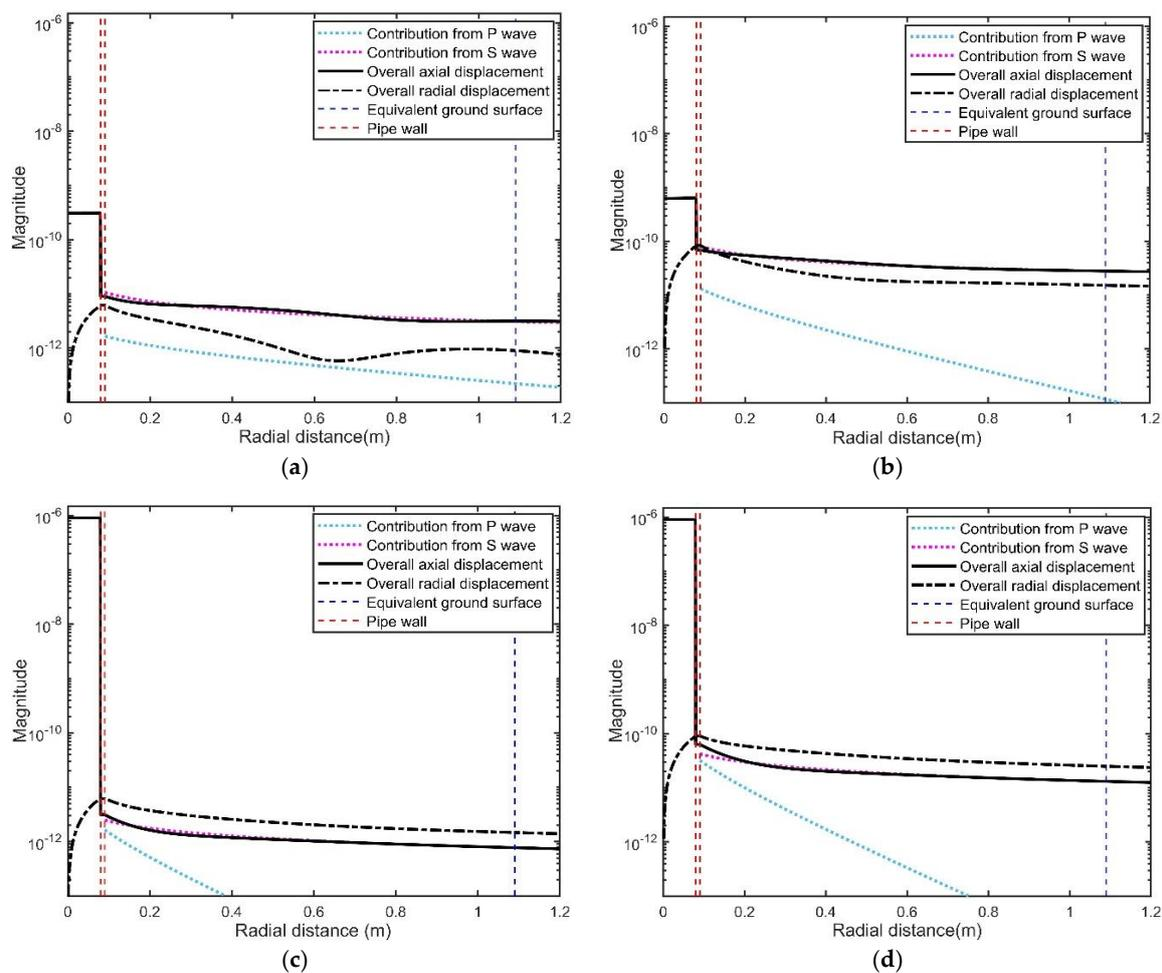
**Figure 6.** Displacement profiles in radial direction resulting from  $s = 1$  waves, for the pipes buried in soil B: (a) cast iron water pipe; (b) PVC water pipe; (c) cast iron gas pipe; and (d) PVC gas pipe.
