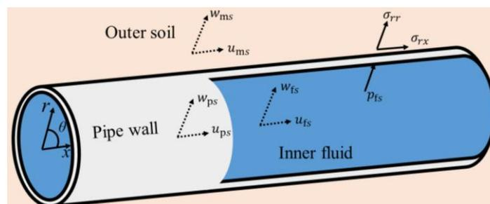
**Figure 1.** The coordinate system for a fluid-filled pipe surrounded by infinite medium.
