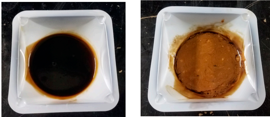
Figure 14. Photographs of downstream oil. The black oil (left) before the change in relative permeability. Brown frothy oil (right) is the produced oil (with CO 2 exsolved) during the relative permeability changes around 40% to 60% CO 2 saturation.
