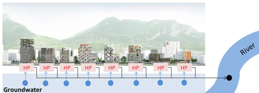
Figure 1. Illustration of the district thermal fed by a groundwater source.
