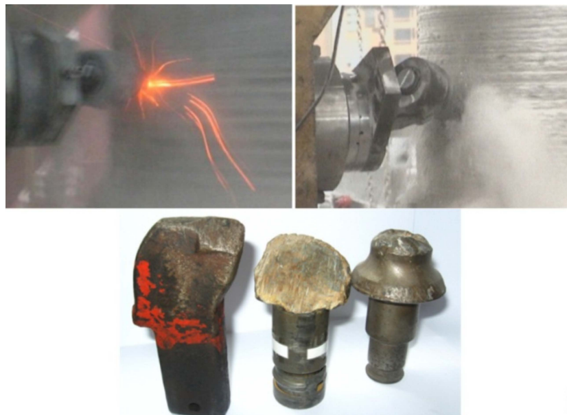
Figure 4. Image of frictional sparking and dust during cutting of a rock sample with a point-rotary-tangential and of pick-wedge wear [5].
