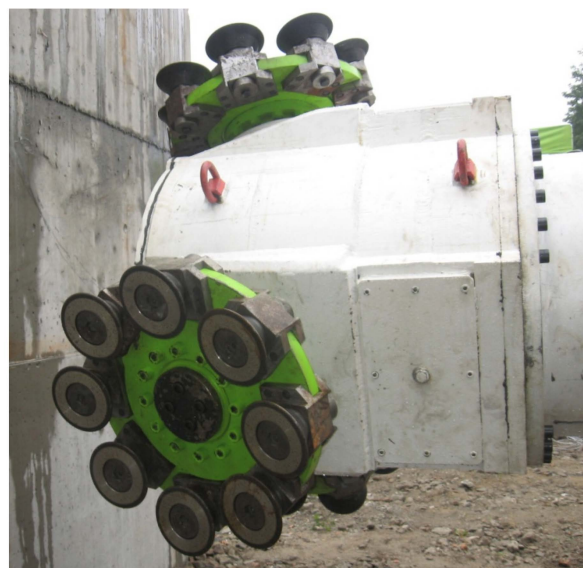
Figure 28. A view of the new mining head solution with complex-trajectory disc tools, ready before field tests.
