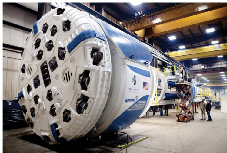
Figure 25. Mining head with disc tools of Robbins TBM [37].
