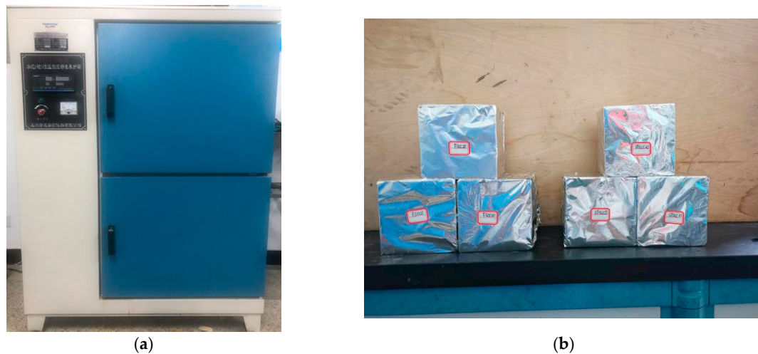
Figure 6. (a) Standard curing. (b) Tinfoil wrapping curing.
