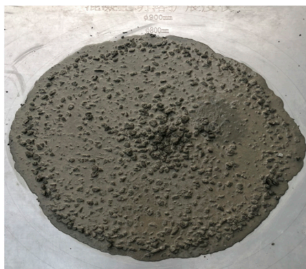
Figure 5. The extending properties of self-compacting concrete (SCC).
