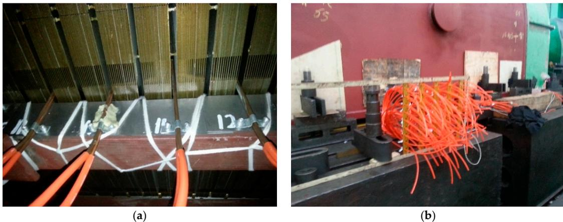
**Figure 2.** Placement and measuring position of pitot tube in the stator ventilation ducts. (a) Placement position of pitot tube; (b) measuring position of ventilation duct.
