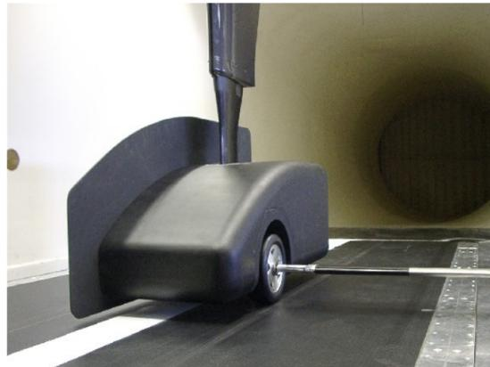
Figure 5. Experimental model by Cazat and Gilliéron [17].
