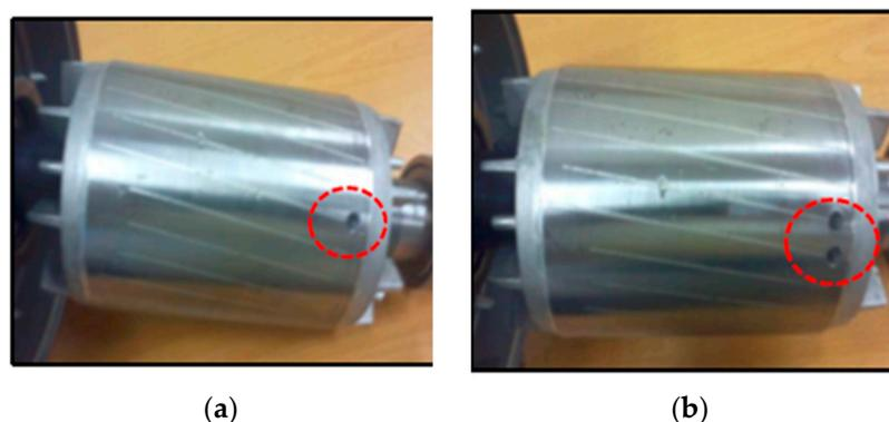
Figure 5. The different induction motors with (a) 1 BRB, and (b) 2 BRBs fault.
