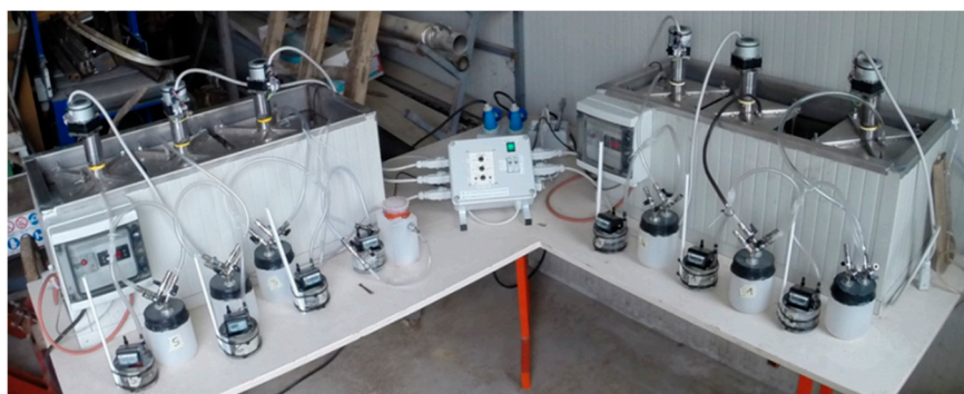
Figure 2. Detail of the experimental anaerobic digestion system.
