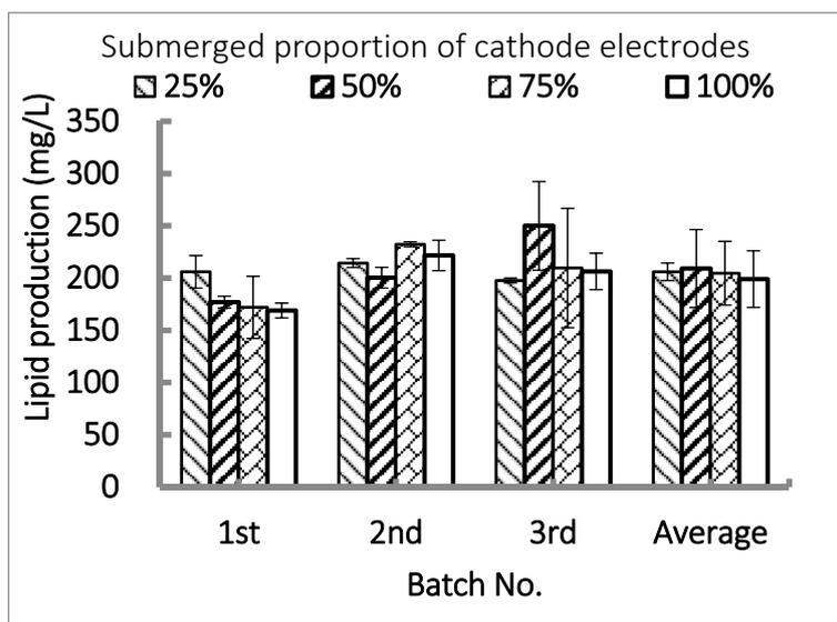
**Figure A1.** Lipid production of microalgae from wastewater with partially and completely submerged electrodes in the cathode chamber.
