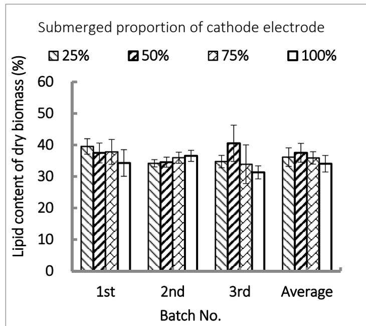
**Figure A2.** Lipid content of dry microalgae biomass from wastewater with partially and completely submerged electrodes in the cathode chamber.
