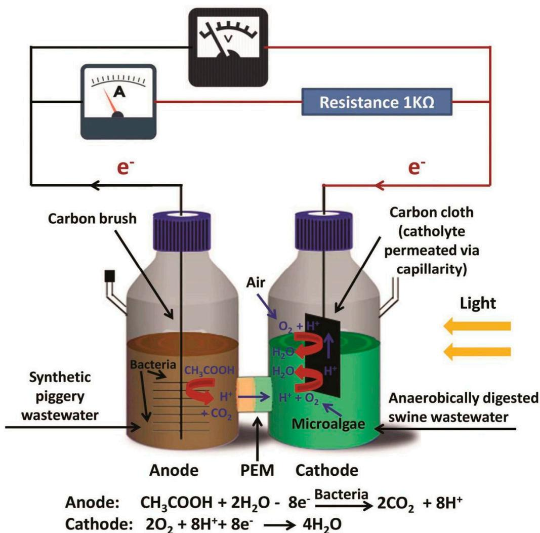
Figure 1. Configuration of the microbial fuel cell (MFC) reactor.
