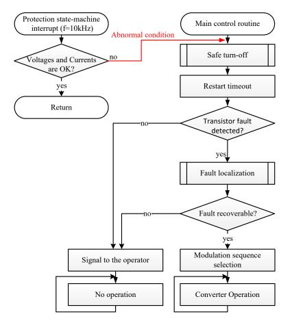
Figure 2. Generalized fault detection procedure for the case study current source converter.
