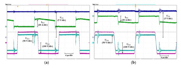
Figure 8. Operating waveforms in the FBK-SMC mode: boost (a) and buck (b).  $U_{CS} = 24$  V, P = 300 W.
