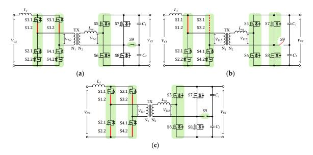
**Figure 3.** Reconfiguration possibilities of the case study converter: asymmetric secondary-modulated converter (A-SMC): (**a**), flyback secondary-modulated converter (FBK-SMC) (**b**), and symmetric secondary-modulated converter (S-SMC) (**c**).
