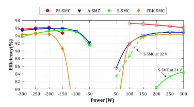
**Figure 9.** Measured efficiencies in different operating modes at  $U_{CS} = 24$  V (unless otherwise specified); negative power values denote buck mode, positive-boost mode.
