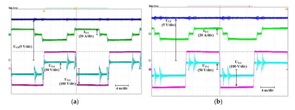
Figure 5. Operating waveforms in the PS-SMC mode: boost (a) and buck (b).  $U_{CS} = 24 \text{ V}, P = 300 \text{ W}.$
