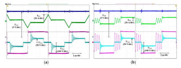
Figure 7. Operating waveforms in the S-SMC mode: boost (a) and buck (b).  $U_{CS} = 24 \text{ V}, P = 300 \text{ W}.$
