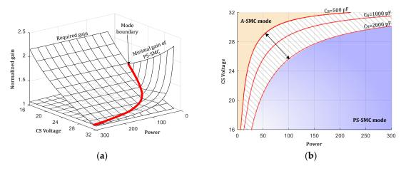
**Figure 4.** Derivation of the borderline between PS- and A-SMC modes for  $C_s = 1$  nF (**a**); theoretical mode boundaries for various  $C_s$  values (**b**).
