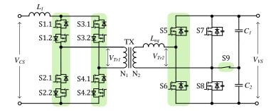
Figure 1. Analyzed PS-SMC converter topology with a reconfigurable rectifier.
