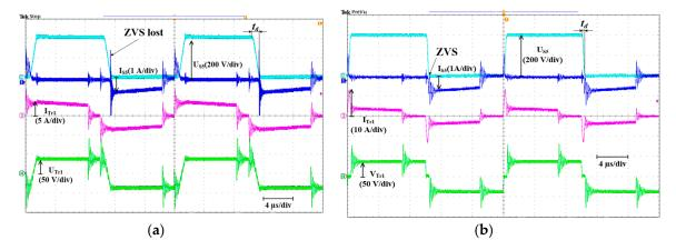
**Figure 11.** Operation in the PS-SMC mode demonstrating the loss of zero-voltage switching (ZVS) (**a**); operation in the A-SMC mode with reduced recharge time  $t_d$  (**b**).  $U_{CS} = 24$  V,  $P_{CS} = 80$  V.
