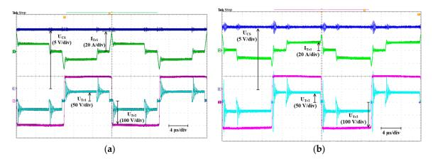
Figure 6. Operating waveforms in the A-SMC mode: boost (a) and buck (b).  $U_{CS} = 24 \text{ V}, P = 300 \text{ W}.$
