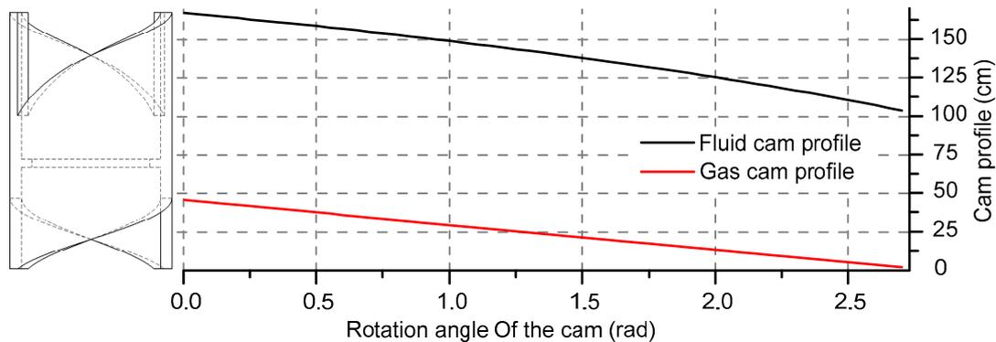
**Figure 5.** Real cam profiles of the new accumulator in the experiments.
