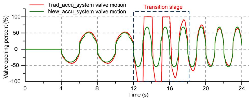
**Figure 10.** Comparison of the valve motions of the two systems when the sine signal frequency suddenly increases from 0.25 Hz to 0.5 Hz.
