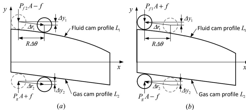
Figure 4. Model of the cam mechanism in 2D: (a) charging process; (b) discharging process.
