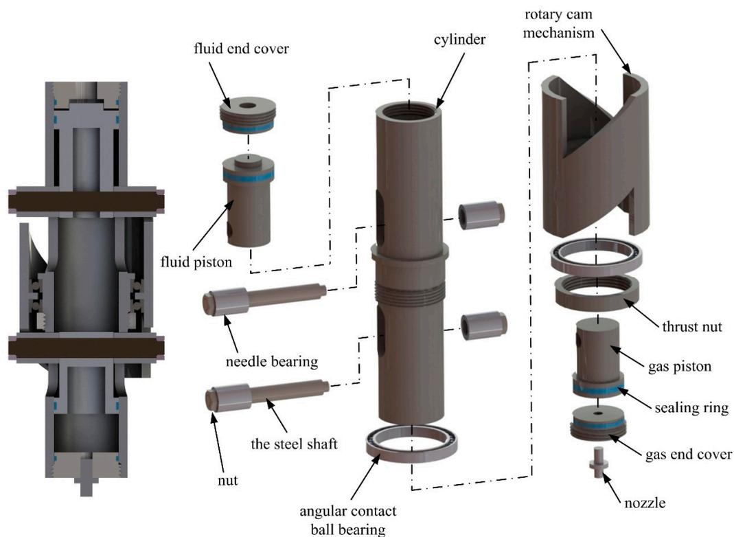
Figure 3. Mechanism structure of the new accumulator.
