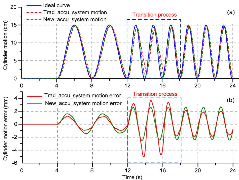
**Figure 11.** Cylinder motion comparisons of the two systems when the sine signal frequency suddenly increases from 0.25 Hz to 0.5 Hz: (a) cylinder motions of the two systems; (b) tracking errors of the two systems.
