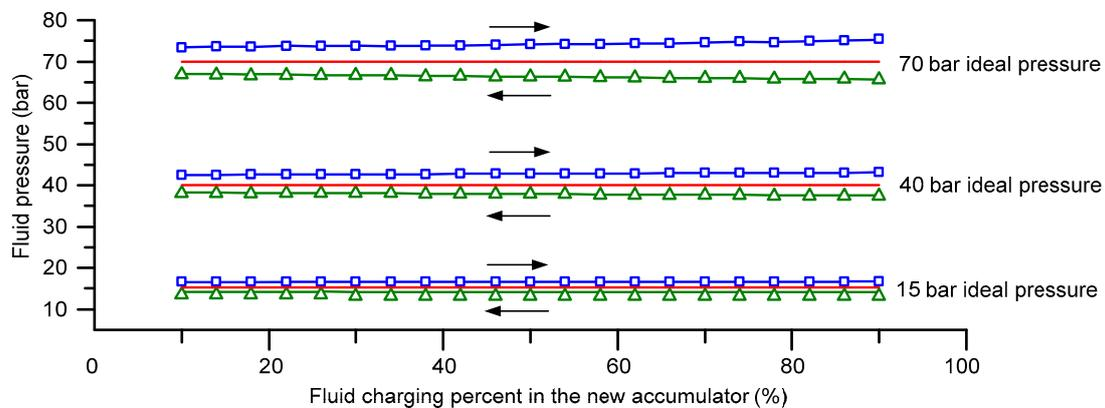
**Figure 8.** The fluid pressure of the new accumulator with a 0.02 m/s piston speed.
