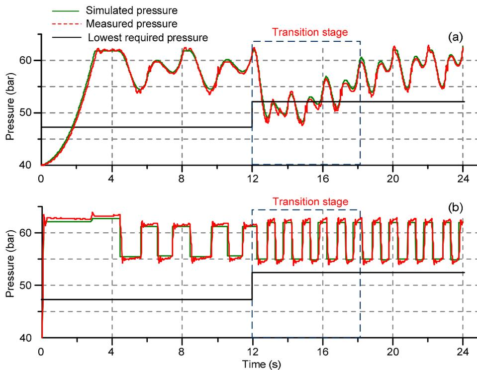
**Figure 9.** Comparison of two pressures of the two accumulator systems when the sine signal frequency suddenly increases from 0.25 Hz to 0.5 Hz: (a) pressure of the traditional accumulator; (b) pressure of the new accumulator.
