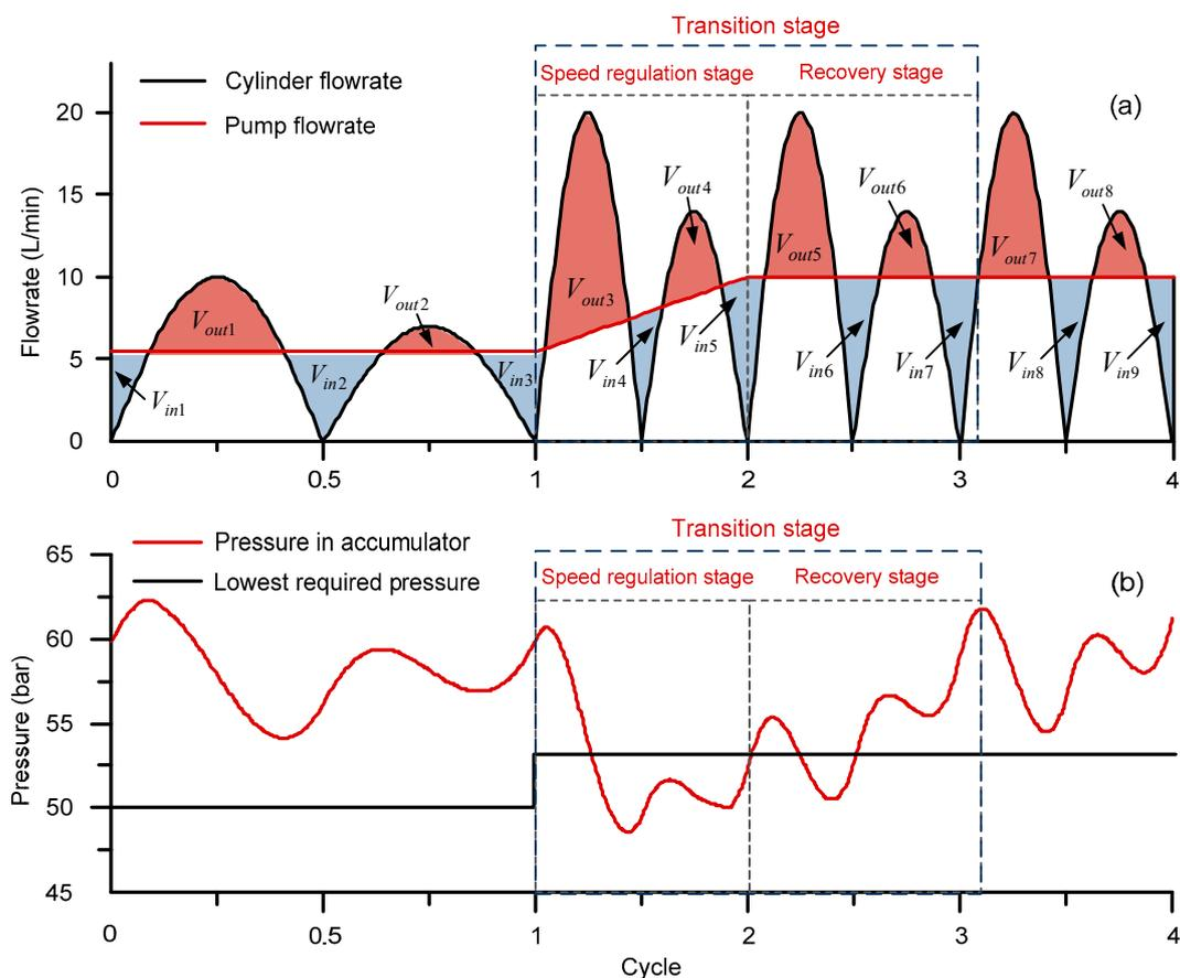
**Figure 2.** Performance of a traditional accumulator in a single cylinder hydraulic system when the working frequency is suddenly doubled: (a) flow rate of the pump and the cylinder; (b) oscillation of the accumulator pressure and the lowest required pressure.
