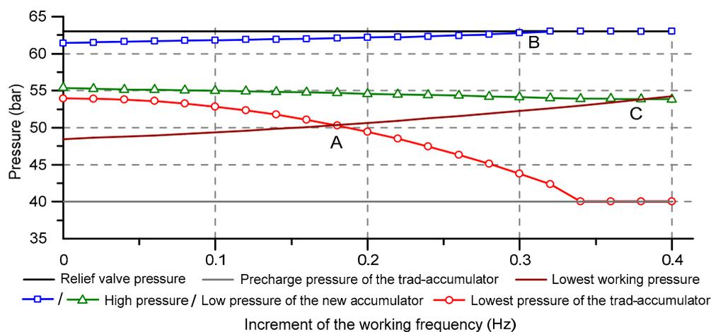
**Figure 12.** Pressure variations of the two accumulators with different increment of the working frequency.
