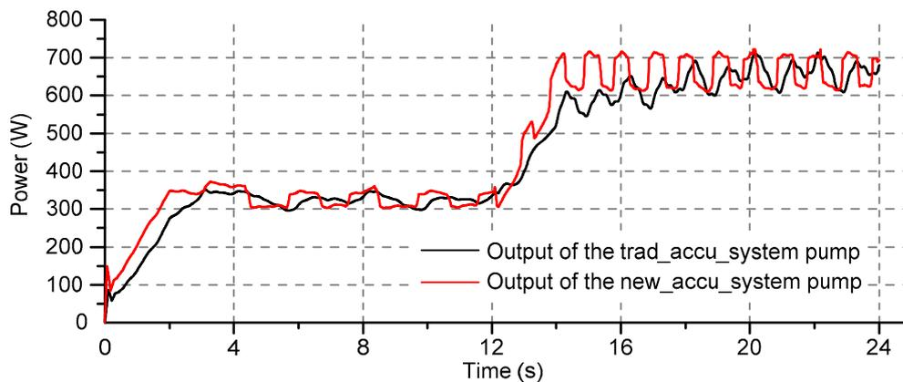
Figure 13. Energy out of the pump in the two systems.
