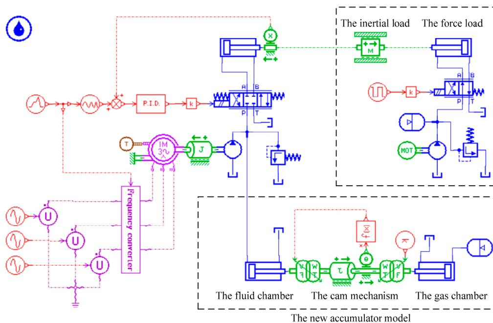
Figure 6. Simulation model constructed on Amesim.
