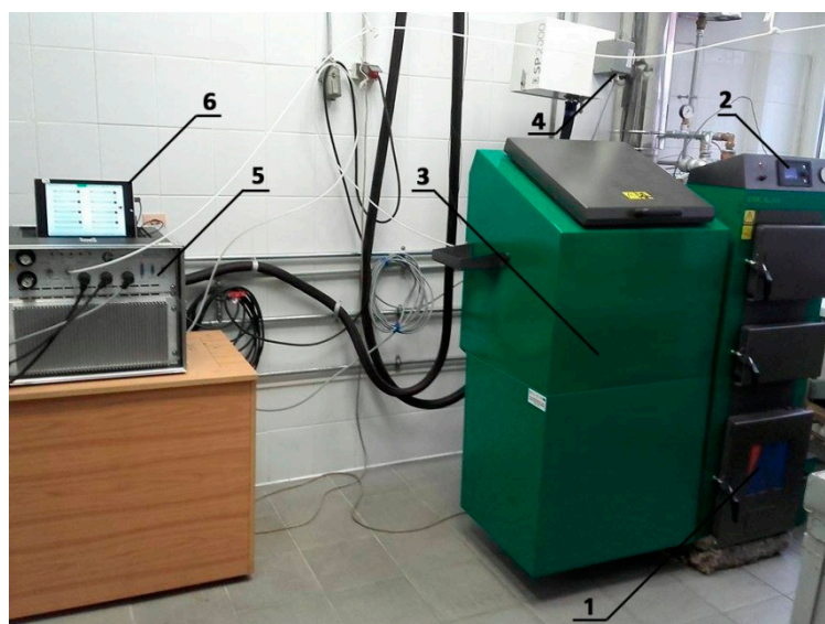
Figure 4. Laboratory stand at Low Emission Combustion Technologies: 1—Moderator Unica VentoEko boiler, 2—boiler controller, 3—fuel tank, 4—exhaust sampling, 5—MCA10 analyzer, 6—Microsoft tablet for archiving measurement results.
