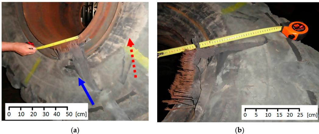
**Figure 5.** Damaged tyre; (a) a part of the tyre that slipped out from the ring; (b) the measurement of the main rupture surface.
