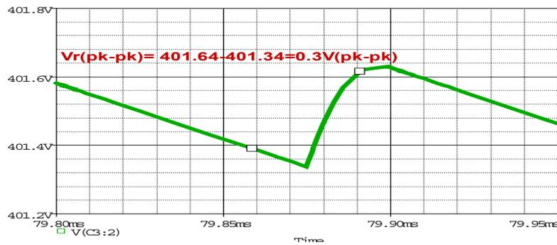
Figure 25. Magnitude of output voltage ripples for [7].
