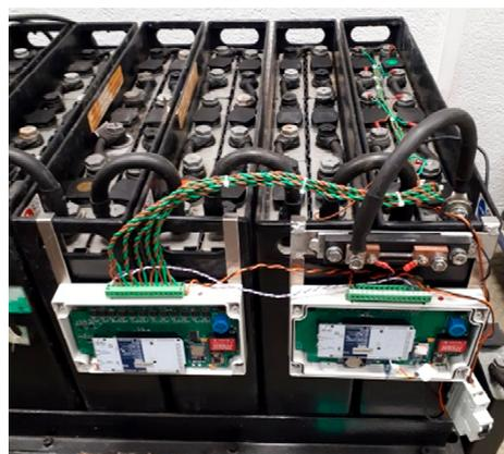
**Figure 6.** Implementation in a battery.
