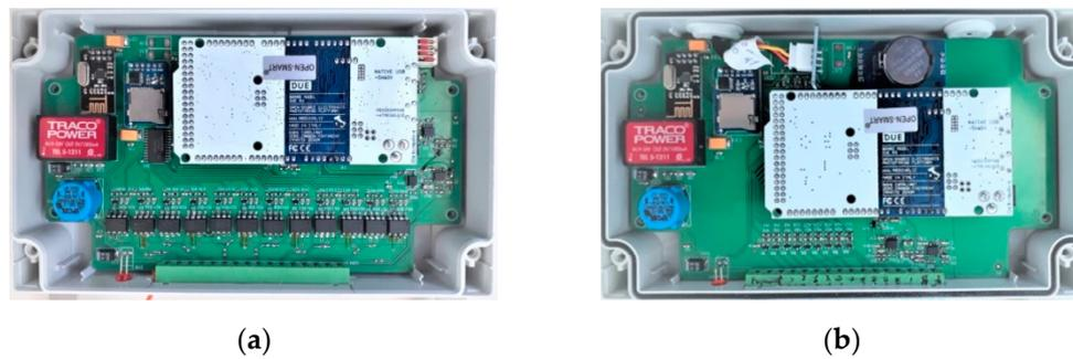
**Figure 4.** (a) Capture unit; (b) Master unit.
