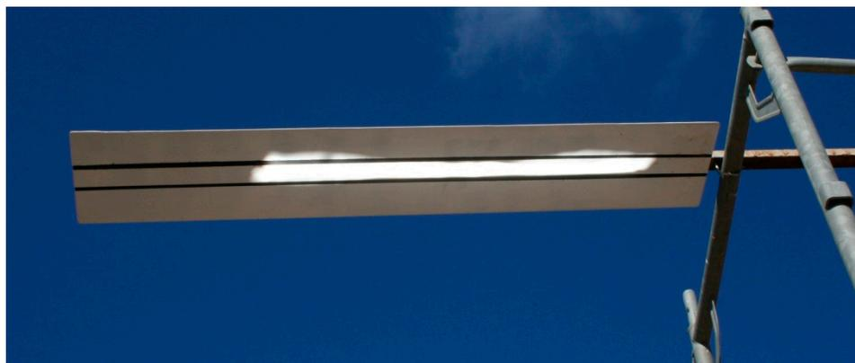
**Figure 12.** Concentrated radiation reflected into a Lambertian target.
