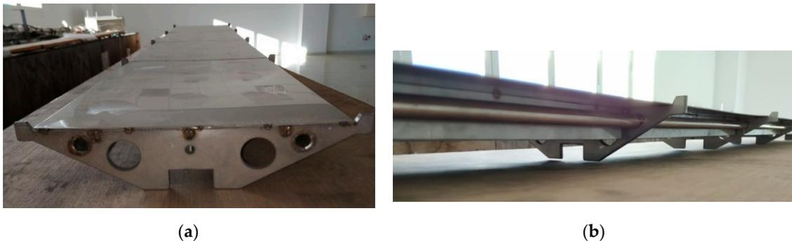
**Figure 6.** Assembly of a curved rectangular plate attached to a set of preformed ribs: (a) front view of the assembly and (b) lateral (longitudinal) view of the assembly.
