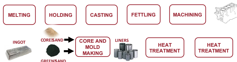
Figure 7. Process flow for Al-alloy engine block manufacturing.
