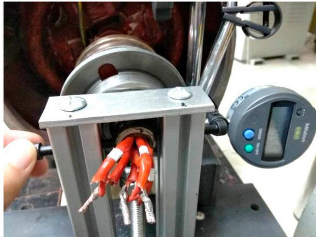
**Figure 7.** Eccentricity adjustment mechanism.
