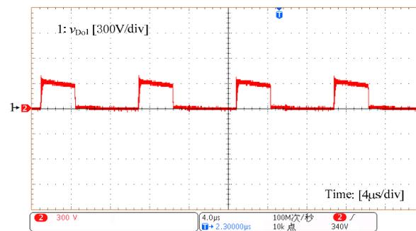
Figure 9. Waveform of  $v_{D01}$ .
