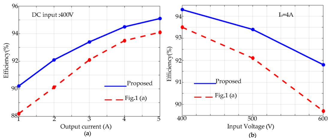
Figure 12. Efficiency curves: (a)  $V_{in} = 400V$ ,  $I_o$  is varied; (b)  $I_o = 4A$ ,  $V_{in}$  is varied.
