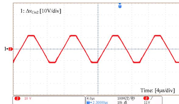
Figure 8. Waveform of  $\Delta v_{Cin2}$ .
