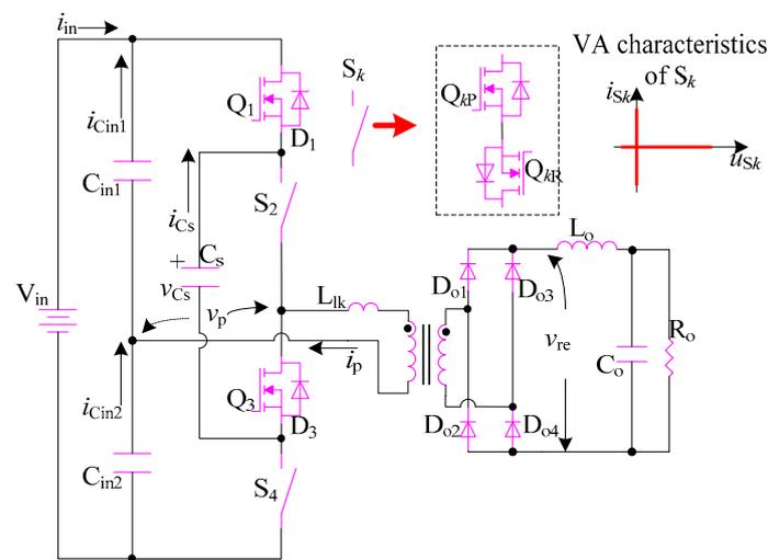
Figure 2. Proposed capacitor-clamped ZVZCS HB TLDC.
