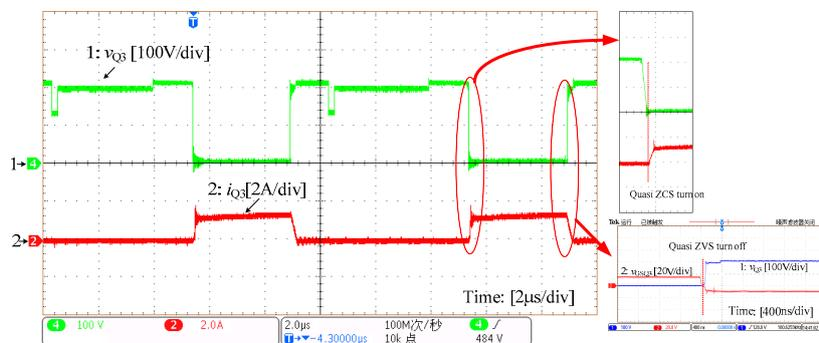
Figure 11. Waveform of  $v_{Q3}$ ,  $i_{Q3}$  and  $v_{GSQ3}$ .
