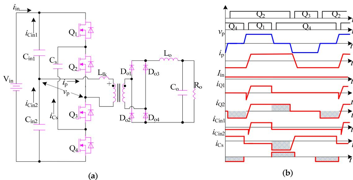
**Figure 1.** Capacitor-clamped HB TLDC and its key waveforms: (a) Circuit; (b) Key waveforms.
