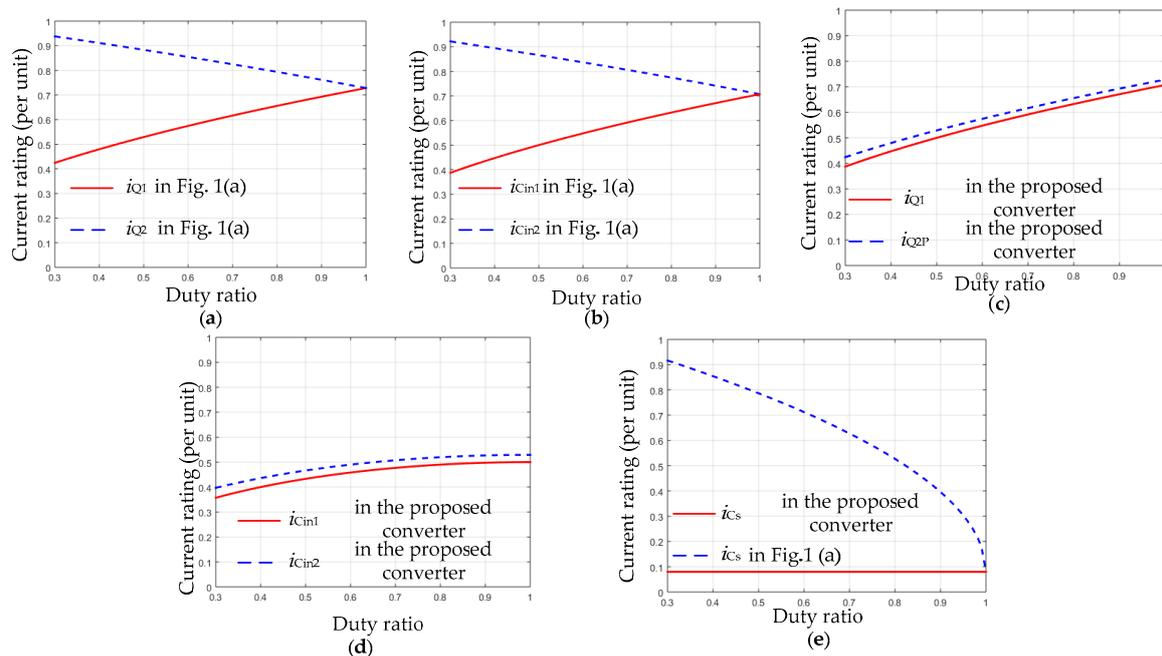
**Figure 5.** Current of the primary switches: (a)  $i_{Q1}$  and  $i_{Q2}$  in Figure 1a; (b)  $i_{C_{in1}}$  and  $i_{C_{in2}}$  in Figure 1a; (c)  $i_{Q1}$  and  $i_{Q2P}$  in the proposed converter; (d)  $i_{C_{in1}}$  and  $i_{C_{in2}}$  in the proposed converter; (e)  $i_{C_s}$ .
