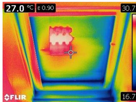
**Figure A3.** Illustrative infrared picture of a roof window. A multiple reflection of a heating body is clearly visible, which affects the window, in particular the radiative heat transfer component.
