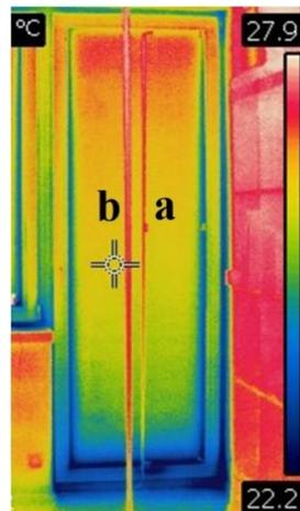
**Figure A2.** Illustrative infrared picture of a glazed balcony door. **a:** a thin textile ribbon installed 15 mm in front of the glazing surface; **b:** a thin textile ribbon at a distance of 1.4 m from the glazing. Both ribbons were used for indirect informative measurement of the temperature of the surrounding air.
