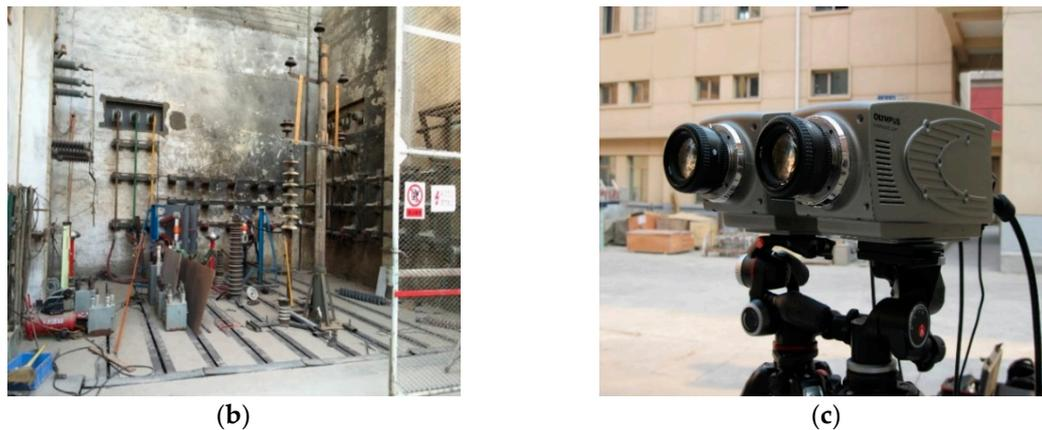
**Figure 4.** Experimental platform for secondary arc reproduction: (a) Experimental circuit; (b) experiment field; (c) high-speed cameras.
