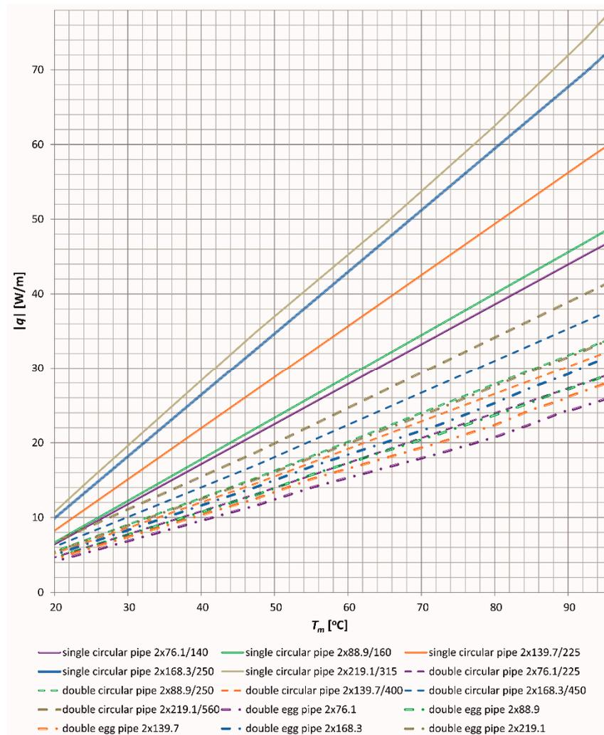
**Figure 5.** Unit heat loss for different types of pre-insulated pipes as a function of the average supply and return temperature of the heating medium for the studied heating network in northeastern Poland.
