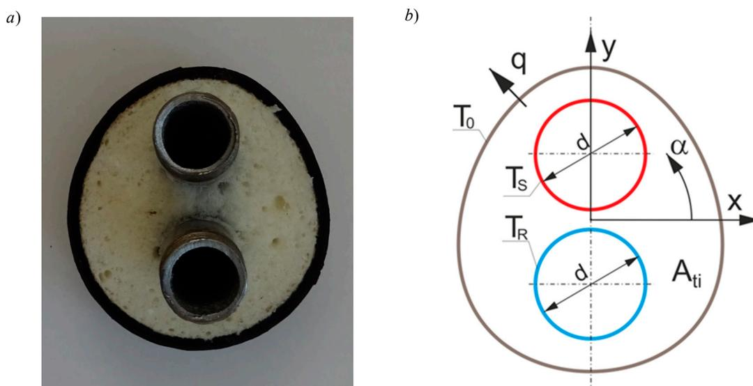
**Figure 1.** An example of a prototype (a) of a double pre-insulated, egg-shaped thermal insulation pipe made as part of the VIPSKILLS 2016-1-PL01-KA203-026152 project Erasmus+, and boundary conditions (b) adopted for calculating numerical heat losses in the adopted double heating networks.
