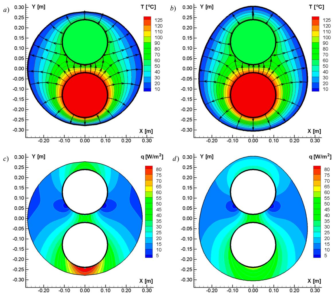
**Figure 2.** Temperature field with heat lines (a,b) and heat flux density (c,d) for the double pre-insulated duct in circular (a,c) and egg thermal insulation (b,d) ( $T_S = 130$  °C,  $T_R = 55$  °C).
