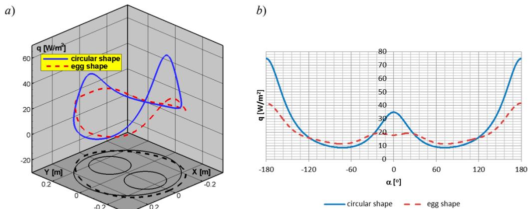
**Figure 3.** Distribution of the heat flux density at the boundary of the cross-section of the thermal insulation of round shape (blue solid line) and egg shape (red dotted line): (a)  $q = f(x,y)$ ; (b)  $q = f(\alpha)$ .
