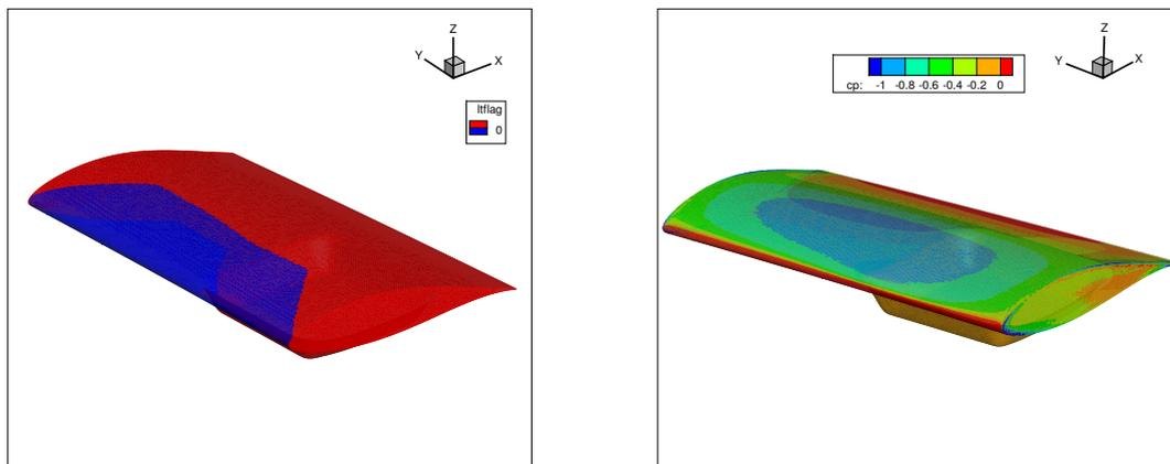
**Figure 10.** (Left): Estimated flow state regions from 3D transitional computational fluid dynamics (CFD), DLR -TAU code). (Blue) Laminar flow; (Red) fully turbulent flow. (Right): Static pressure coefficient.
