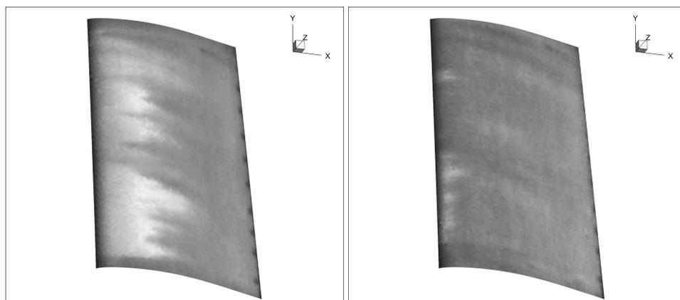
**Figure 18.** Thermal images from Figure 17 after reconstruction and mapping onto the 3D grid of the aerodynamic glove. Images are from 11:22:27 (Left) and 11:23:13 (Right), both SCADA time. Here, only the glove is shown.
