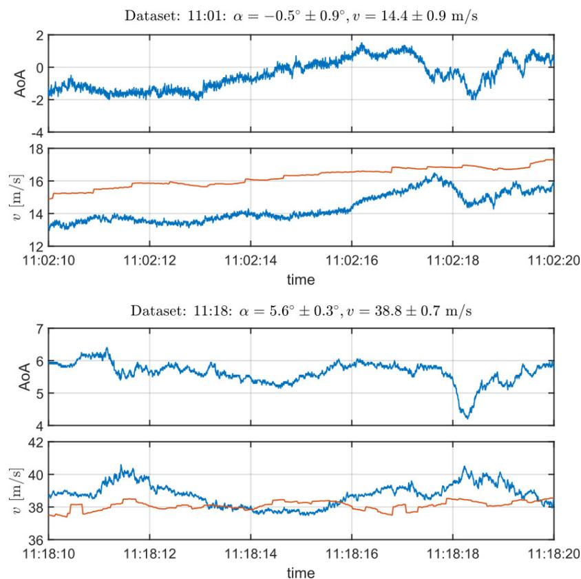
**Figure 11.** Inflow properties of different operation states. (**Top**) Start-up (SU); (**Bottom**) steady state (SS). Shown are AOA (**Upper row**) and inflow velocity (**Lower row**). (**Blue**) Velocity obtained by five-hole probe; (**Red**) velocity obtained by SCADA data.
