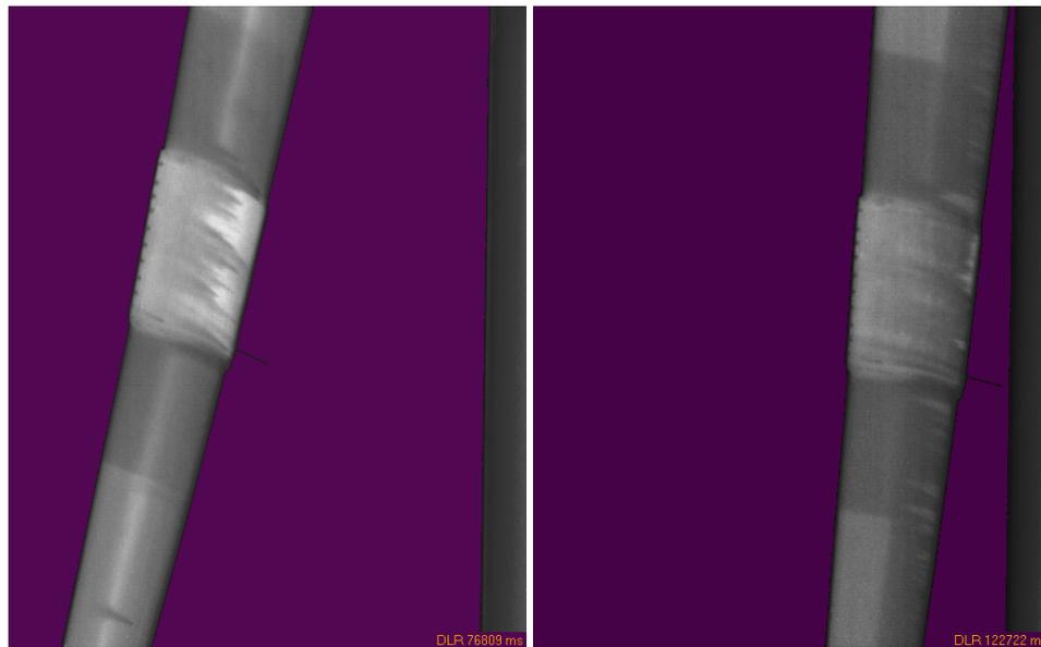
**Figure 17.** Two typical thermal images obtained by DLR setup after image processing including bad-pixel elimination, sky-background replacement, and contrast enhancement. Images are from 11:22:27 (Left) and 11:23:13 (Right), both SCADA time. Left shows more laminar parts during startup, and right only very small extended regions during constant rpm (approximately 9) operation mode.
