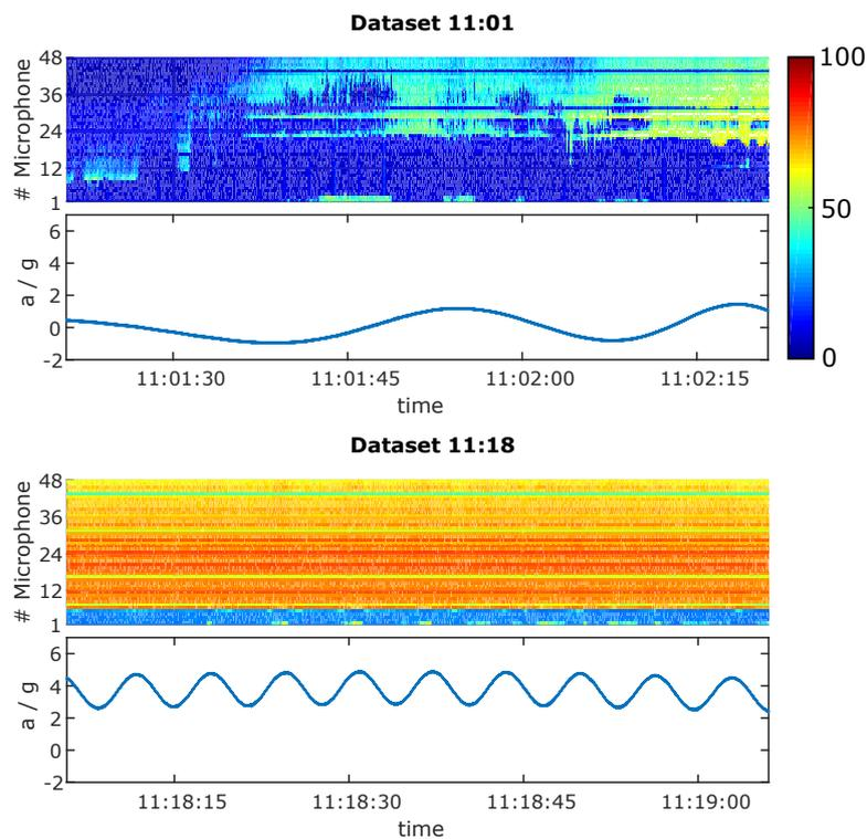
**Figure 13.** Detection of the transition position. (Top) SU; (Bottom) SS. (Upper row) Sound-pressure level (SPL) in Decibels (dB). (Color map) Dark blue corresponds to 0 dB and red to 80 dB. (Lower row) Local acceleration.
