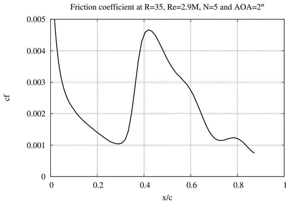
**Figure 8.** Location of transition from wall shear stress ( $c_f$ ) by CFD code FLOWer.  $N = 5$  corresponds to a TI ( $TI$ ) of 0.3%. Onset of transition may be located at  $x/c = 0.29$ , and flow is fully turbulent at  $x/c = 0.42$ . Slope is at maximum at  $x/c = 0.36$ .
