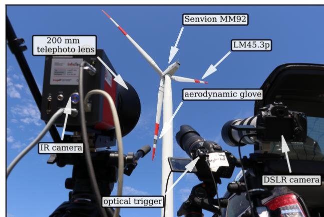
**Figure 5.** Experimental setup for thermographic flow visualization measurements. Foreground: thermographic camera with 200 mm telephoto lens, optical trigger, and DSLR camera for documentation purposes.
