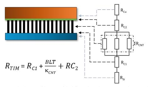
**Figure 3.** Simple schematic of the origin of the different thermal resistance contributions in the CNT array TIM. The black contributions were included in the thermal interface resistance results that were obtained from the laser flash experiment [15].
