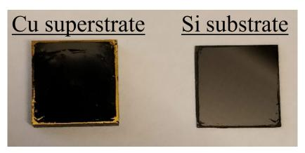
**Figure 6.** Shearing of the CNT array TIMs always resulted in a delamination where the CNTs remained on the Cu superstrate side leaving the Si substrate with a clean surface.
