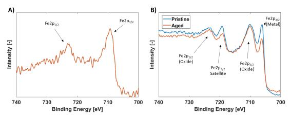
**Figure 8.** XPS analysis results of the Fe peak: (A) from the roots of the CNTs remaining on the Cu superstrate after delamination; and (B) from the Si substrate after delamination before and after thermal aging.
