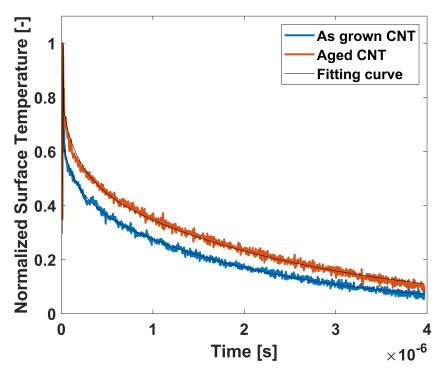
**Figure 7.** Time—temp response curve from PPR measurements on samples before and after thermal aging together with the numerical fitting curves.
