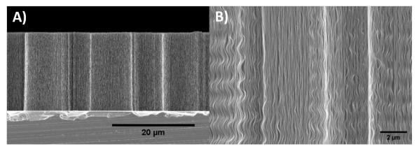
**Figure 2.** (**A**) Side view SEM image of a CNT array grown on a silicon substrate using the CVD process; and (**B**) high magnification view of the CNT array, which resolves the individual strands.
