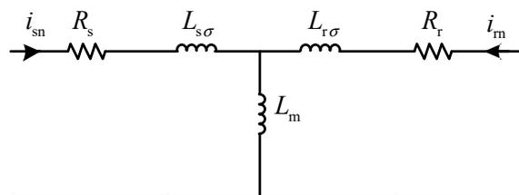
Figure 4. Equivalent circuit of the DFIG.
