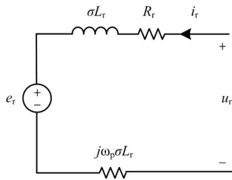
Figure 2. Rotor equivalent circuit of the DFIG.
