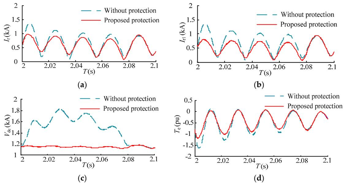
**Figure 14.** Response of proposed protection under a voltage sag of 0.6. (a) Rotor current; (b) RSC current; (c) DC-link bus voltage; and (d) electromagnetic torque.
