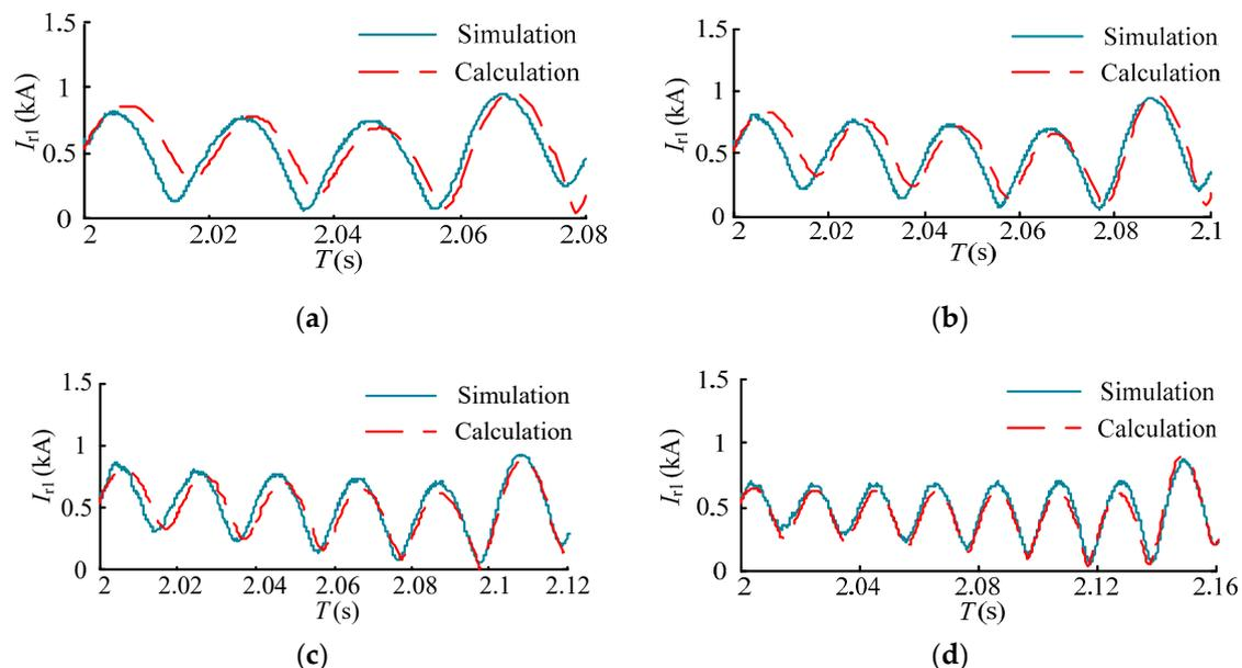
Figure 13. Comparison between calculation and simulation. (a) Voltage sag of 0.5; (b) voltage sag of 0.6; (c) voltage sag of 0.7; and (d) voltage sag of 0.8.
