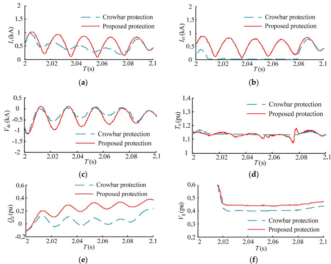
**Figure 16.** Comparisons between proposed protection and crowbar protection under a voltage sag of 0.6. (a) Rotor current; (b) RSC current; (c) electromagnetic torque; (d) DC-link bus voltage; (e) reactive power at the grid; and (f) the terminal voltage.
