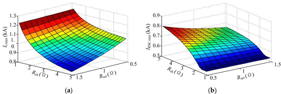
**Figure 9.** Calculation results under different parameters. (a) The maximum of the rotor current; and (b) the maximum of the RSC current.
