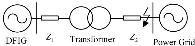
Figure 12. Simulation model of the DFIG.
