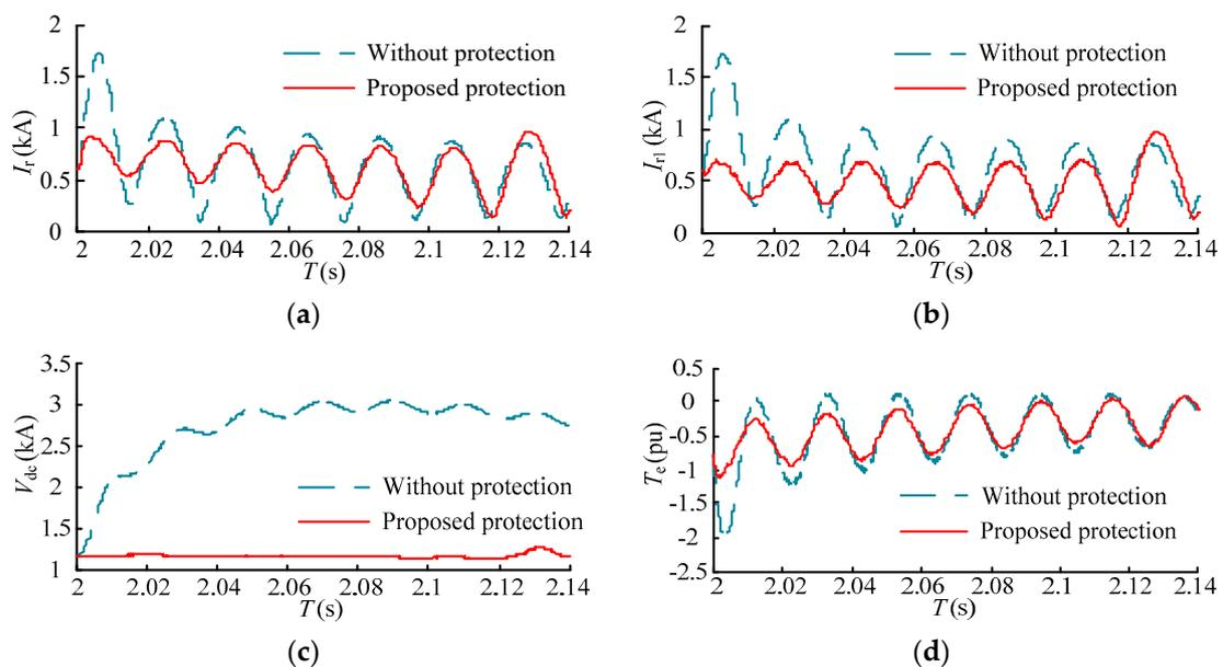
**Figure 15.** Response of proposed protection under a voltage sag of 0.8. (a) Rotor current; (b) RSC current (c) DC-link bus voltage; and (d) electromagnetic torque.
