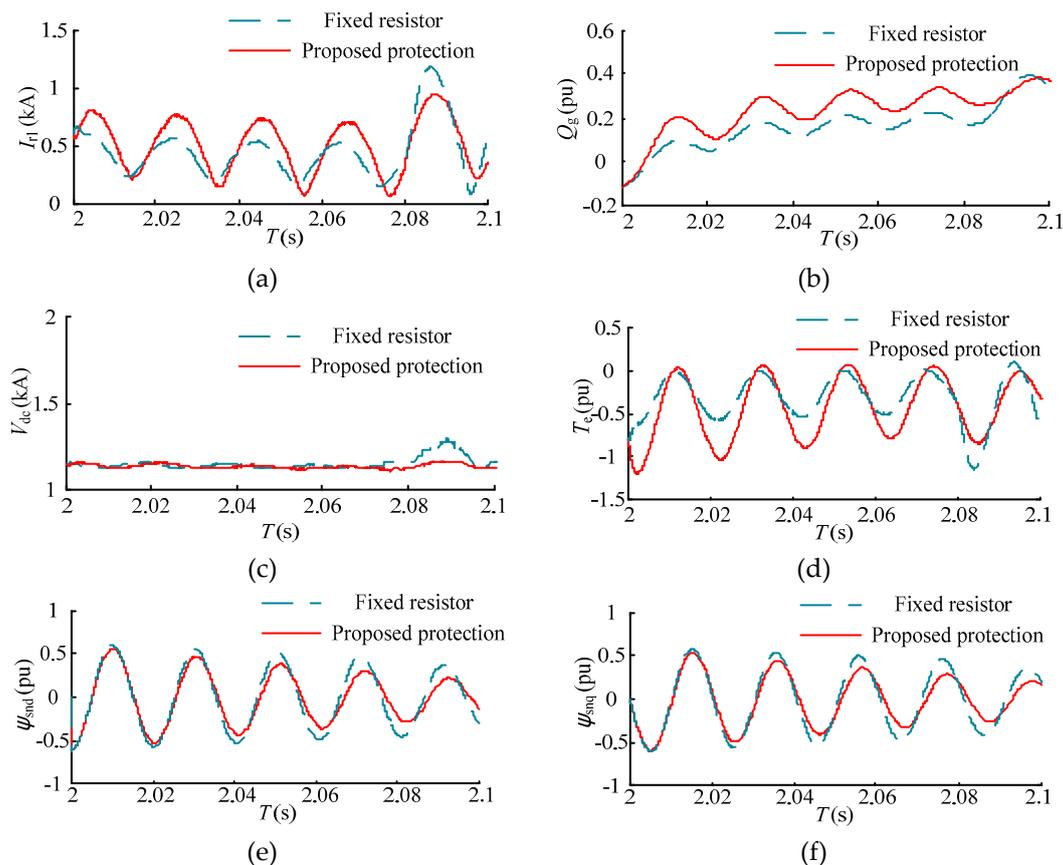
**Figure 20.** Comparison between proposed protection and fixed rotor braking resistor. (a) RSC current; (b) reactive power at the grid; (c) DC-link bus voltage; (d) electromagnetic torque; (e) the D-axis component of the stator transient flux linkage; and (f) the Q-axis component of the stator transient flux linkage.
