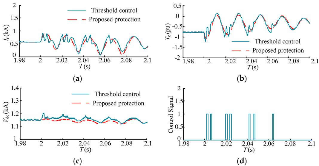
**Figure 18.** Comparisons between proposed protection and threshold control under a voltage sag of 0.6. (a) Rotor current; (b) electromagnetic torque; (c) DC-link bus voltage; and (d) the control signal of rotor braking resistor.
