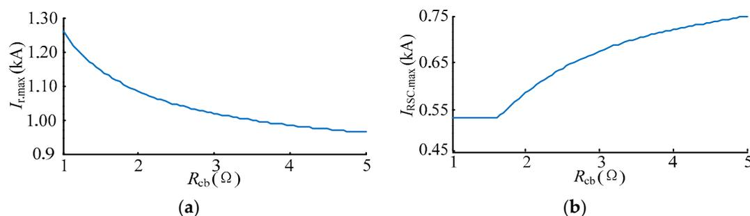
**Figure 10.** Calculation results under different crowbar resistors. (a) The maximum of the rotor current; and (b) the maximum of the RSC current.
