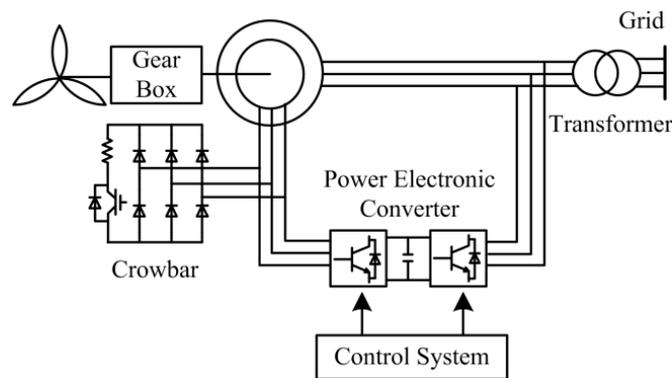
Figure 1. Structure of wind turbine driven by a DFIG.
