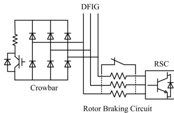
Figure 3. Configuration of the proposed protection.
