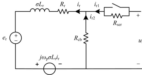
Figure 7. Rotor equivalent circuit of the DFIG.
