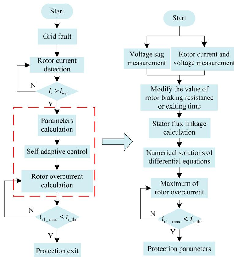
Figure 11. Flow diagram of the self-adaptive control.
