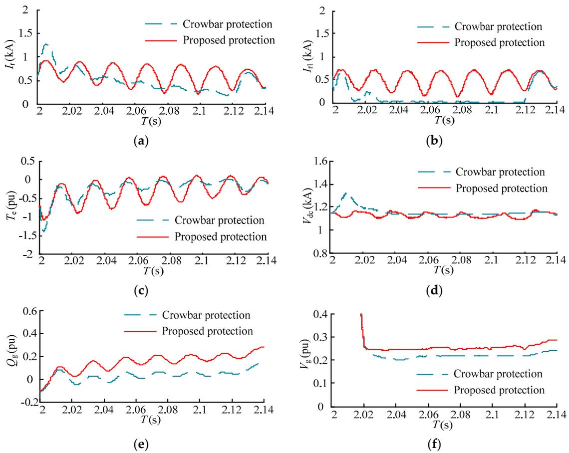
**Figure 17.** Comparisons between proposed protection and crowbar protection under a voltage sag of 0.8. (a) Rotor current; (b) RSC current; (c) electromagnetic torque; (d) DC-link bus voltage; (e) reactive power at the grid; and (f) the terminal voltage.
