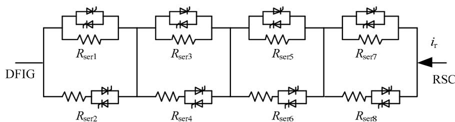
**Figure 6.** Rotor braking resistor array.
