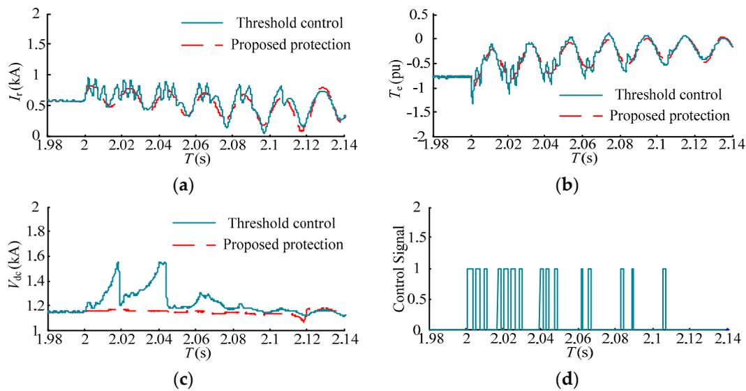
**Figure 19.** Comparisons between proposed protection and threshold control under a voltage sag of 0.8. (a) Rotor current; (b) electromagnetic torque; (c) DC-link bus voltage; and (d) the control signal of rotor braking resistor.
