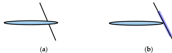
Figure 4. The illustration of crossing between the hydraulic fracture and natural fracture: (a) crossing, and (b) arrested. The oval represents the hydraulic fracture, the thin, black line represents the natural fracture, and the bold, blue line represents the opening natural fracture.
