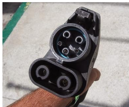
Figure 1. SAE J1772 EV connector standard with DC fast-charging combined charging system (CCS 1) [18].
