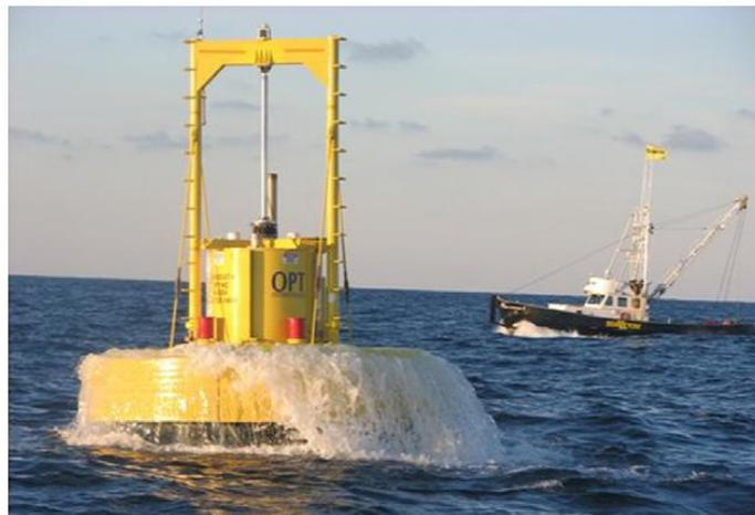
**Figure 2.** The PowerBuoy WEC oscillating in the sea [49].
