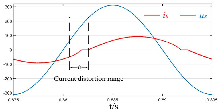
Figure 19. Simulation waveforms of grid voltage and input current when  $i_s$  lags  $u_s$  by  $45^\circ$ .
