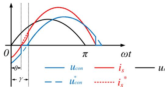
**Figure 9.** Expected waveforms and actual waveforms of AC-side fundamental voltage and current under a lagging power factor ( $U_L > |U_s \sin \theta|$ ).
