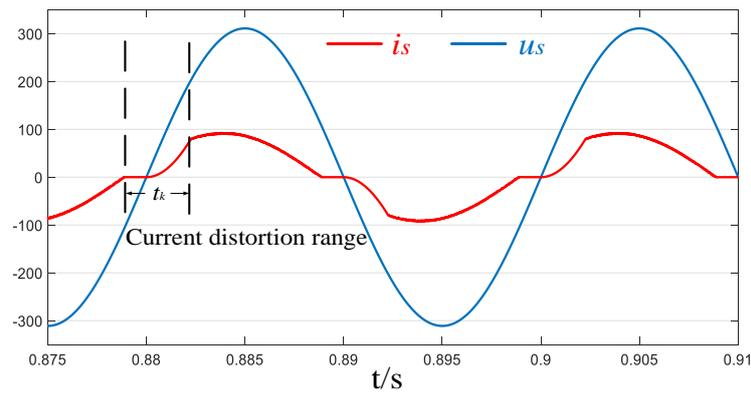
Figure 17. Simulation waveforms of grid voltage and input current under leading power factor.
