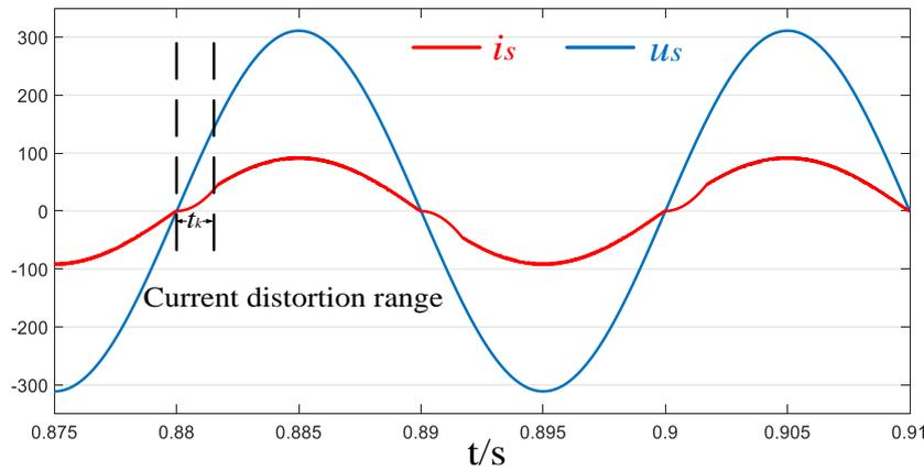
Figure 14. Simulation waveforms of grid voltage and input current under unity power factor.
