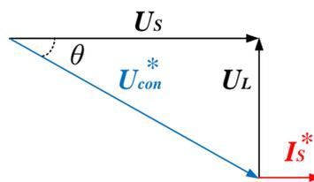
Figure 5. Phasor diagram on the AC side under unity power factor.
