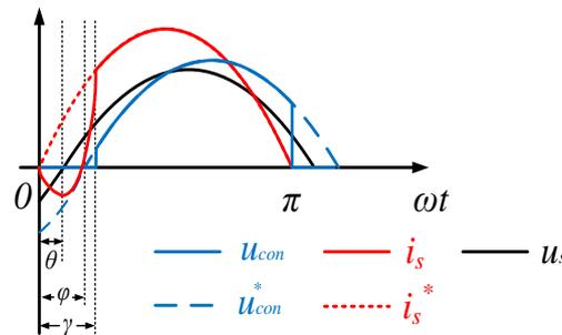
**Figure 7.** Expected waveforms and actual waveforms of the AC-side fundamental voltage and current with synchronous drive under a leading power factor.
