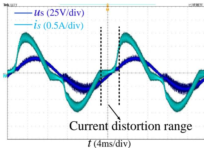
Figure 24. Experiment waveforms of grid voltage and input current under leading power factor.
