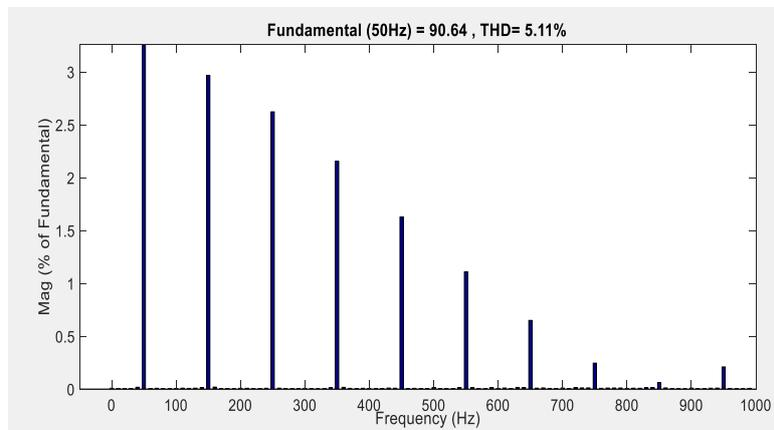
Figure 15. THD analysis of input current under unity power factor.
