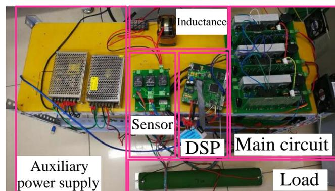
Figure 21. Down-scale experimental prototype.
