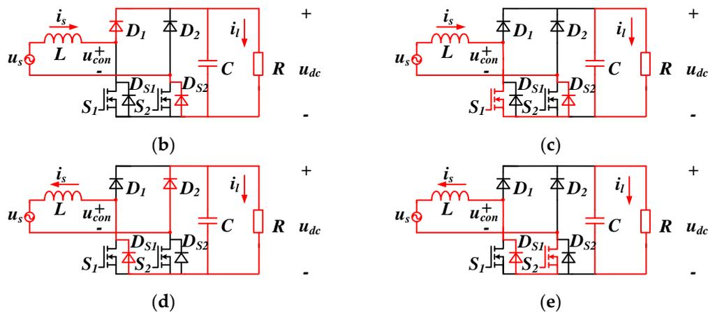
**Figure 1.** Main topology of the bridgeless rectifier and its four operation modes: (a) Main topology of the bridgeless rectifier; (b) Mode I; (c) Mode II; (d) Mode III; (e) Mode IV.
