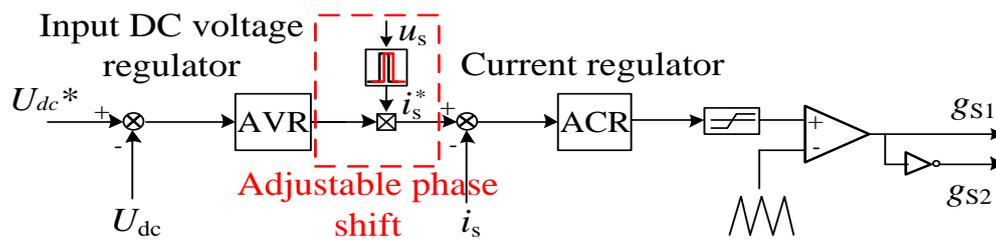
Figure 2. Block diagram of the complementary drive.
