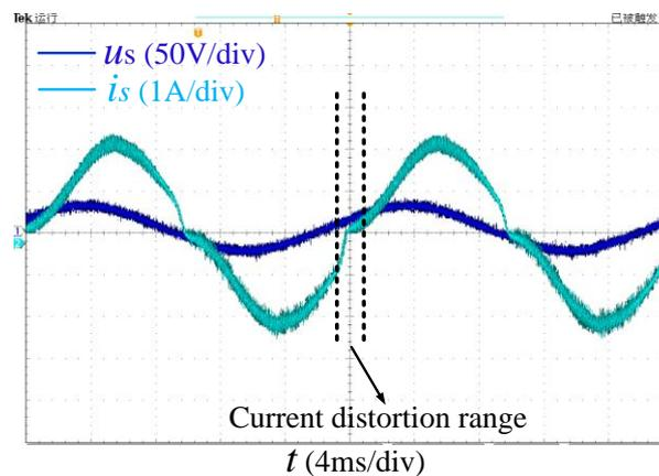
Figure 26. Experiment waveforms of grid voltage and input current when  $i_s$  lags  $u_s$  by  $40^\circ$ .
