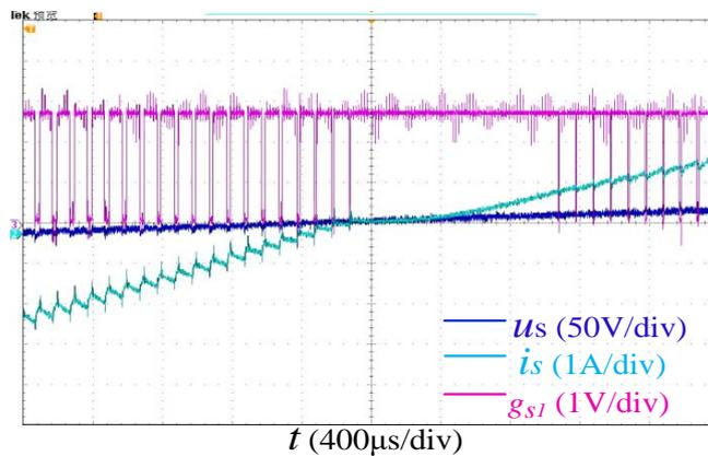
Figure 23. Zoomed-in experiment waveforms of grid voltage and input current under unity power factor.
