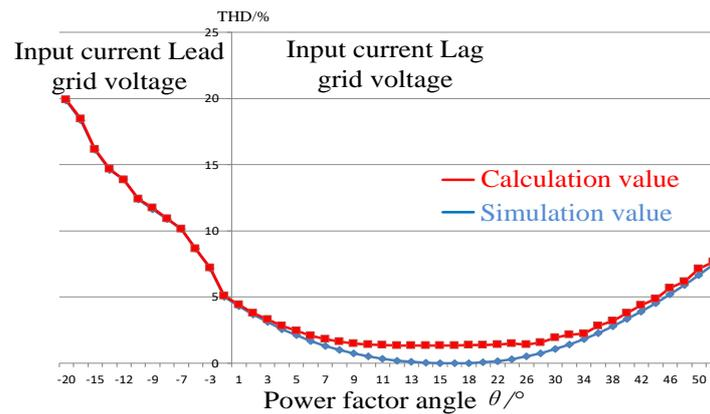
Figure 20. Relationship between theoretical THD and simulation THD with power factor angle  $\theta$ .
