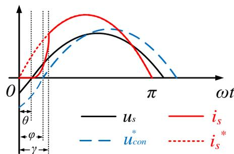
**Figure 8.** Expected waveforms and actual waveforms of AC side fundamental voltage and current with complementary drive under leading power factor.
