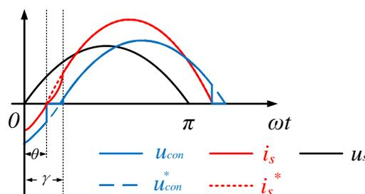
**Figure 10.** Expected waveforms and actual waveforms of AC side fundamental voltage and current under lagging power factor ( $U_L < |U_s \sin \theta|$ ).
