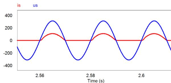
Figure 4. Simulation current waveform on the alternating current (AC) side based on a synchronous drive without an absolute value module.
