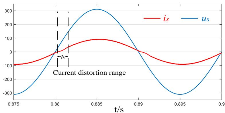
Figure 18. Simulation waveforms of grid voltage and input current when  $i_s$  lags  $u_s$  by  $5^\circ$ .
