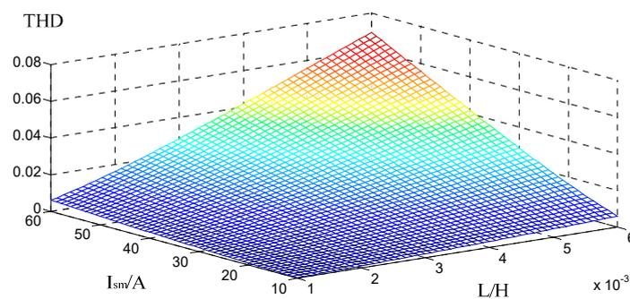
**Figure 11.** Three-dimensional (3D) diagram of current total harmonic distortion (THD) under a unity power factor.
