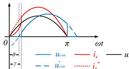
Figure 6. Expected waveforms and actual waveforms of the AC-side fundamental voltage and current of bridgeless rectifier under a unity power factor.
