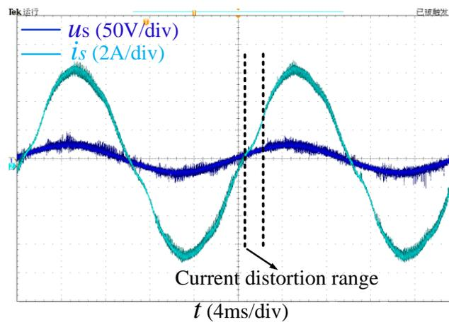
Figure 25. Experiment waveforms of grid voltage and input current when  $i_s$  lags  $u_s$  by  $8^\circ$ .
