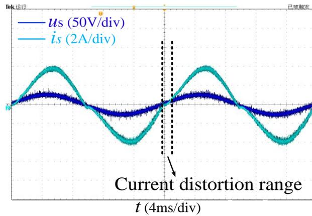
Figure 22. Experiment waveforms of grid voltage and input current under unity power factor.
