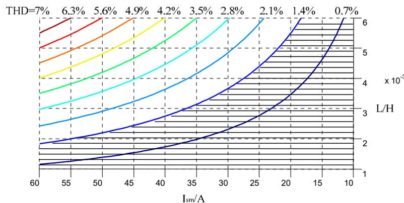
**Figure 12.** Contour line of current THD under a unity power factor.
