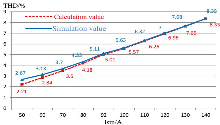
Figure 16. Theoretical and simulation THD under a unity power factor.
