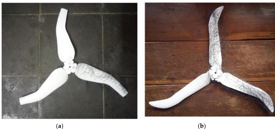
Figure 3. Three-dimensional printed models of the rotors with a radius of 0.19 m. (a) The blade has a backward swept at its tip; (b) the blade has a helicopter-head blade tip.
