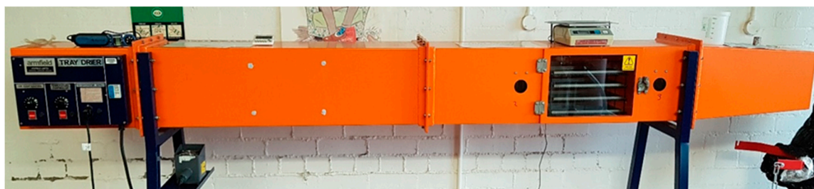
Figure 1. Tray drier working scheme and unit adopted in the experiment.
