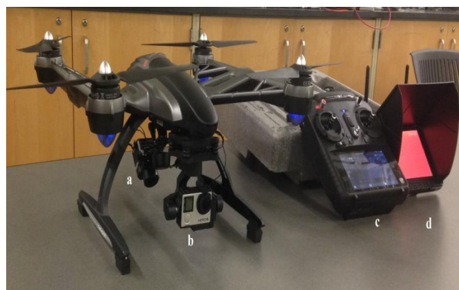
Figure 8. Drone system with thermal and CCD cameras: (a) FLIR Thermal Camera, (b) GoPro CCD Camera, (c) ST-10, and (d) FPV monitor.
