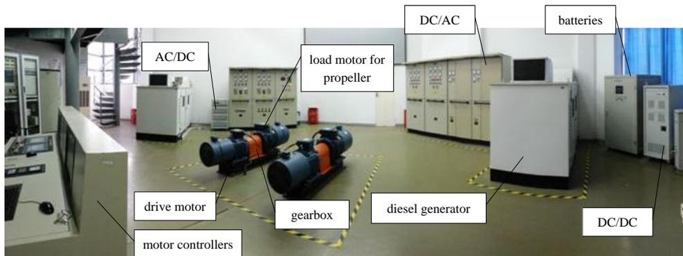
Figure 4. Hybrid ships' experimental platform.
