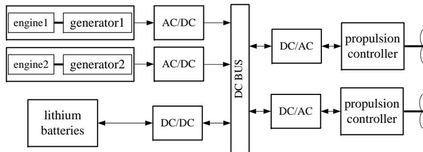
Figure 3. Block diagram of hybrid power ships.
