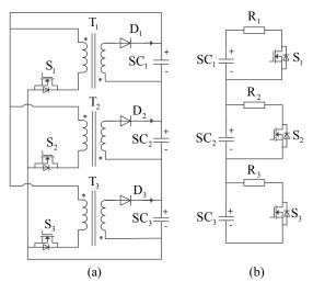
**Figure 24.** Charge and discharge type balancing topology used in the comparative experiment. (a) Charge type in [18]. (b) Discharge type in [22].
