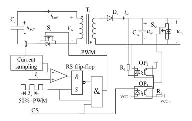
Figure 9. Control circuit of the cascaded converter module.
