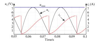
**Figure 15.** Waveform of  $u_0$  and  $i_L$  with the PWM frequency slightly higher than two times of the resonant frequency of *L* and  $C_0$ .
