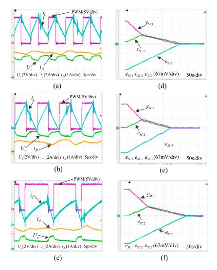
**Figure 23.** The main waveforms of the boost converter and the balancing time. (**a**)–(**c**) are the main waveforms of the boost converter with 2 A, 3.1 A, and 3.6 A average input current, respectively. (**d**)–(**f**) are the corresponding balancing time.
