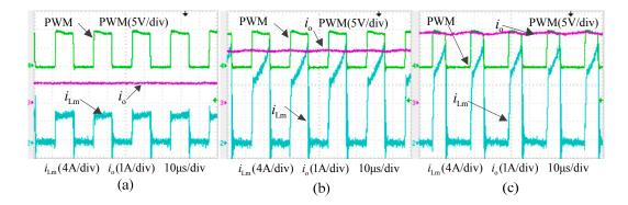
**Figure 20.** Main waveforms of the modularized converter module. (a) With output current  $i_0 = 1$  A. (b) With output current  $i_0 = 3.1$  A. (c) With output current  $i_0 = 4$  A.
