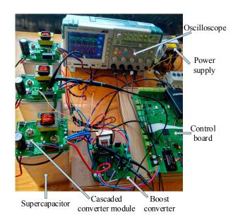
Figure 19. The photograph of the experiment platform.
