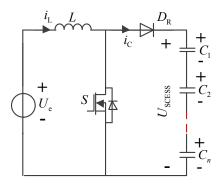
Figure 8. The simplified boost converter.
