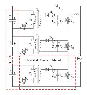
Figure 2. The proposed modularized discharge-type equalizer.
