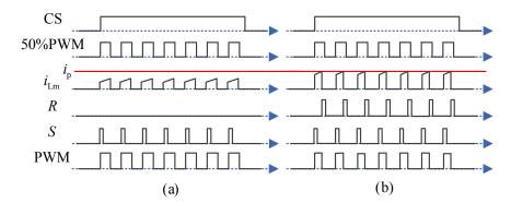
**Figure 10.** Main waveforms of the cascaded converter module. (**a**) With a small load current. (**b**) With a big load current.
