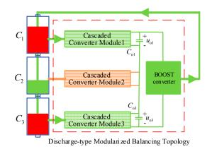
Figure 3. The balancing principle block diagram of the proposed topology.
