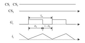
Figure 4. The drive of the cascaded converter modules and the main waveforms of the boost converter.
