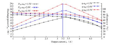
Figure 21. The discharging power and efficiency change with output current.
