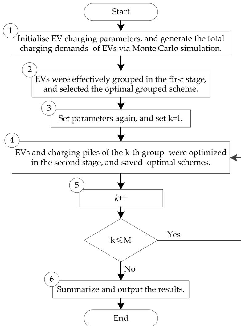
Figure 1. The flowchart of two-stage optimization model.
