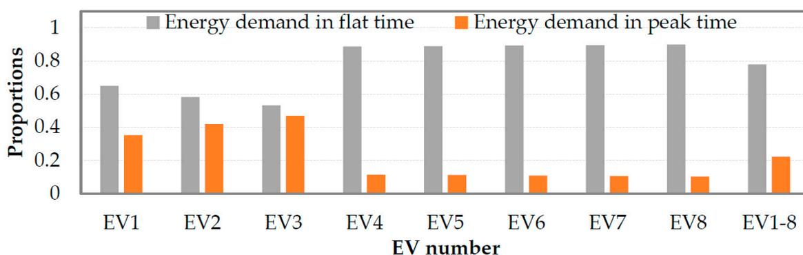
Figure 8. The charge distribution of EVs under OCP.
