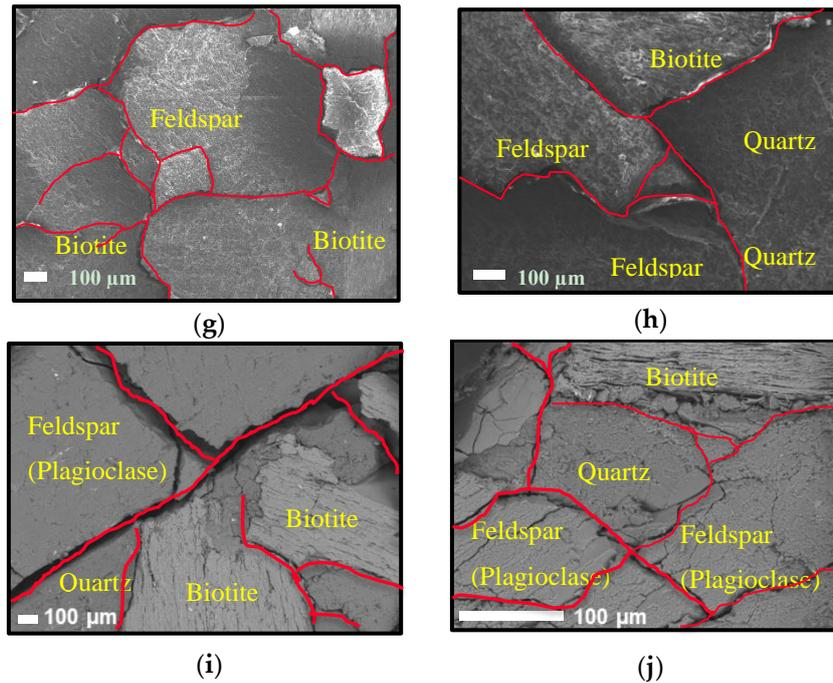
**Figure 5.** SEM images of heat-treated rock slices (a) 100 °C RC, (b) 100 °C SC, (c) 200 °C RC, (d) 200 °C SC, (e) 400 °C RC, (f) 400 °C SC, (g) 600 °C RC, (h) 600 °C SC, (i) 800 °C RC and (j) 800 °C SC where RC denotes Rapid cooling and SC denotes: Slow cooling) Note: SEM image (j) under 800 °C SC was taken under low magnification compared to 800 °C RC (i) to capture a large area as shown in the scale bar.
