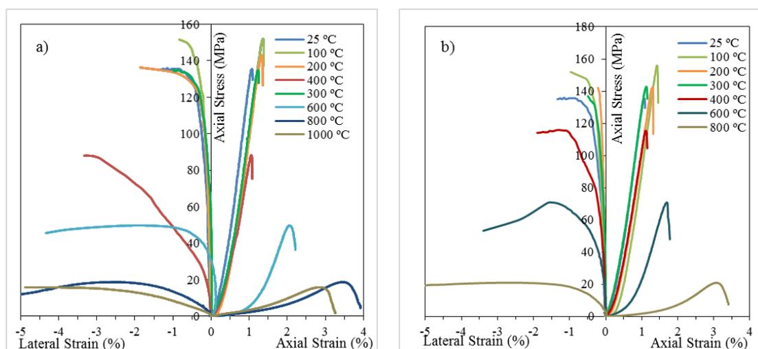
**Figure 7.** Stress-strain curves during axial loading for heat-treated specimens (a) for rapidly cooled specimens (b) for slowly cooled specimens.
