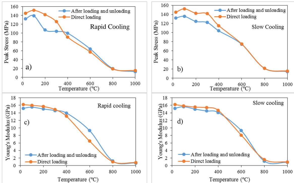
**Figure 12.** Comparison of UCS values and Young's modulus values during direct loading and after loading and unloading cycles for specimens treated with rapid and slow cooling. (a) Peak strength under rapid cooling; (b) Peak strength under slow cooling; (c) Young's modulus under rapid cooling; (d) Young's modulus under slow cooling.
