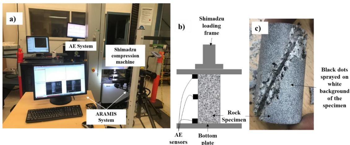
**Figure 4.** Uniaxial compressive strength (UCS) testing set-up (Shimadzu compression machine) with acoustic emission (AE) system and ARAMIS system (a), the sample instrumentation (b), and a tested rock specimen with paint sprayed on the 3-D surface to detect the deformation by tracking co-ordinates (c).
