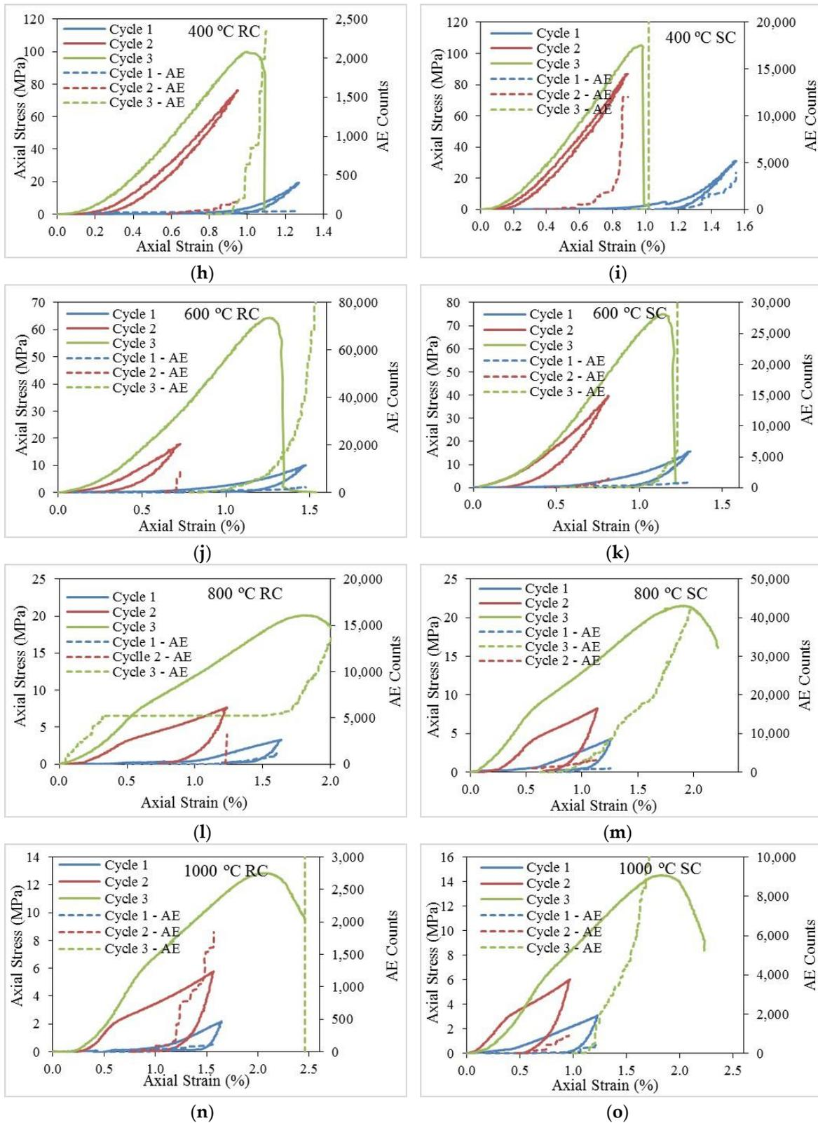
**Figure 11.** Stress-strain curves plotted with AE counts originated during loading and unloading cycles under each test condition, (a) 25 °C; (b) 100 °C RC; (c) 100 °C SC; (d) 200 °C RC; (e) 200 °C SC; (f) 300 °C RC; (g) 300 °C SC; (h) 400 °C RC; (i) 400 °C SC; (j) 600 °C RC; (k) 600 °C SC; (l) 800 °C RC; (m) 800 °C SC; (n) 1000 °C RC; (o) 1000 °C SC where RC denotes rapid cooling and SC denotes slow cooling.
