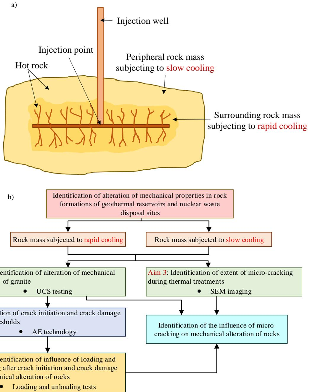
**Figure 3.** (a) Schematic diagram of a hot rock mass which undergoes cooling during fluid injection and (b) the flow of the experimental work covered by the study.
