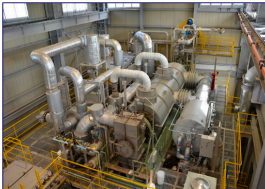
Fig. S1. Outer appearance of the carbonization test facility. The carbonizer (an externally heated rotary kiln) had a diameter of 800 mm (inner cylinder), a length of 6 m, and an effective heating length of 5 m, and it was able to process raw material chips at rates of up to 200 kg/h, although the upper feed rate was dependent on the shape and moisture content of the raw material. The rotation speed of the inner cylinder of the kiln could be controlled to within 1.2–5.5 rpm. The carbonization temperature could be set within a range of 200–650°C by controlling the temperature at the outlet of the blast furnace fueled with liquefied petroleum gas.
